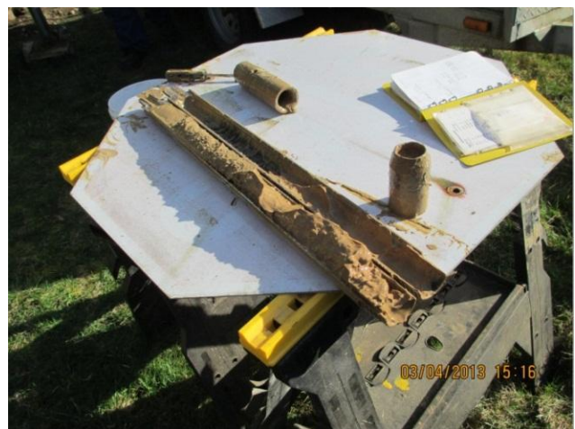
Figure 10. Split spoon sampler from about 15 ft depth
