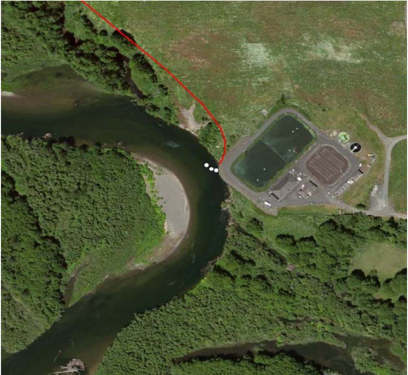
WWTP Vicinity with possible protection alternatives. The sheet pile wall is shown in red, while the piles are shown in the lighter color.
