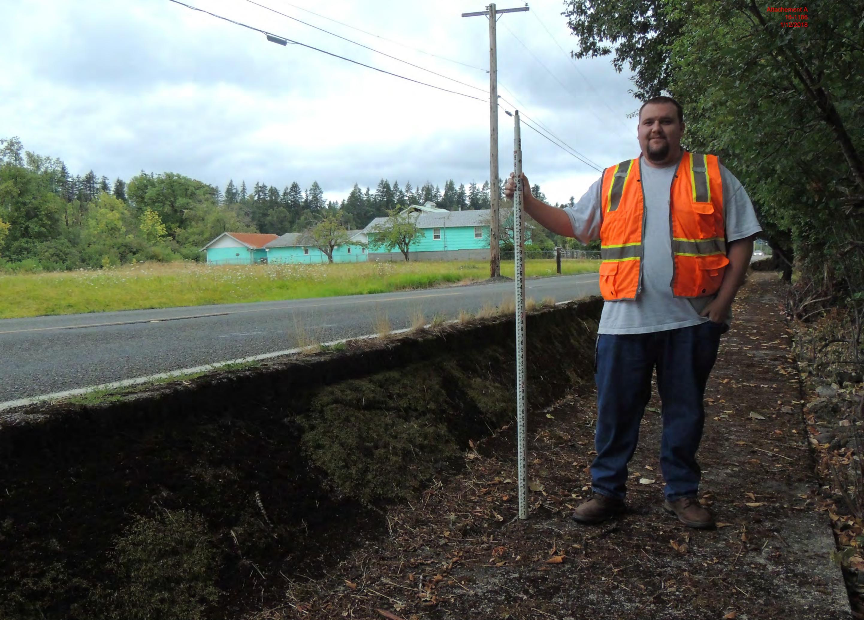
**Flood erosion structure is about 3 ft deep and 5 ft wide, 300 ft long**
