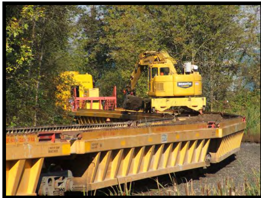
BNSF Track Side Ditch Cleaning Equipment
