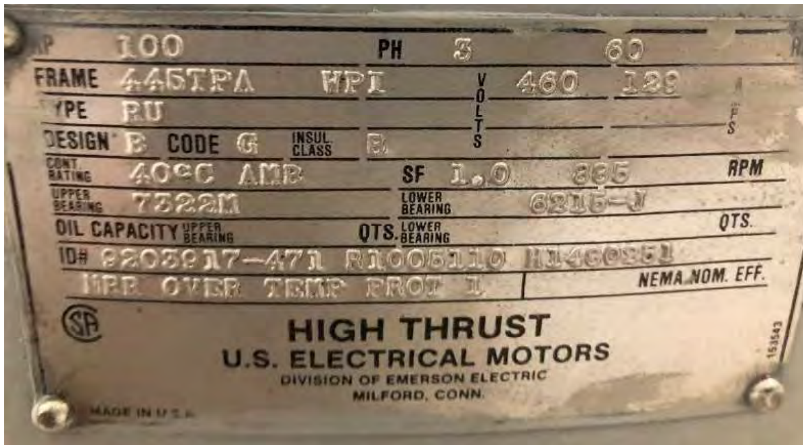
Figure 3-5. 100 hp Pump 2 motor tag
