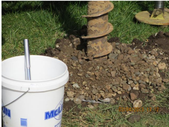
Figure 8. Example of soil materials from about 2-10' depth, loamy sand matrix with periodic layers of clay loam binder
