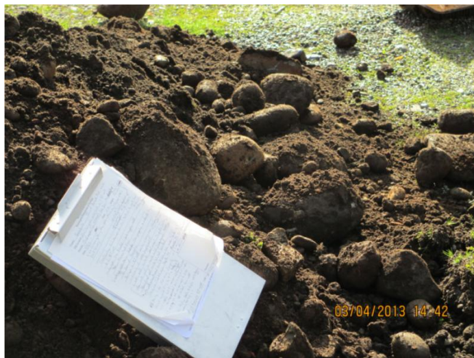
Figure 3. Northern soil pit (SP-1) -- cobbly soils to greater than 7 feet depth.
