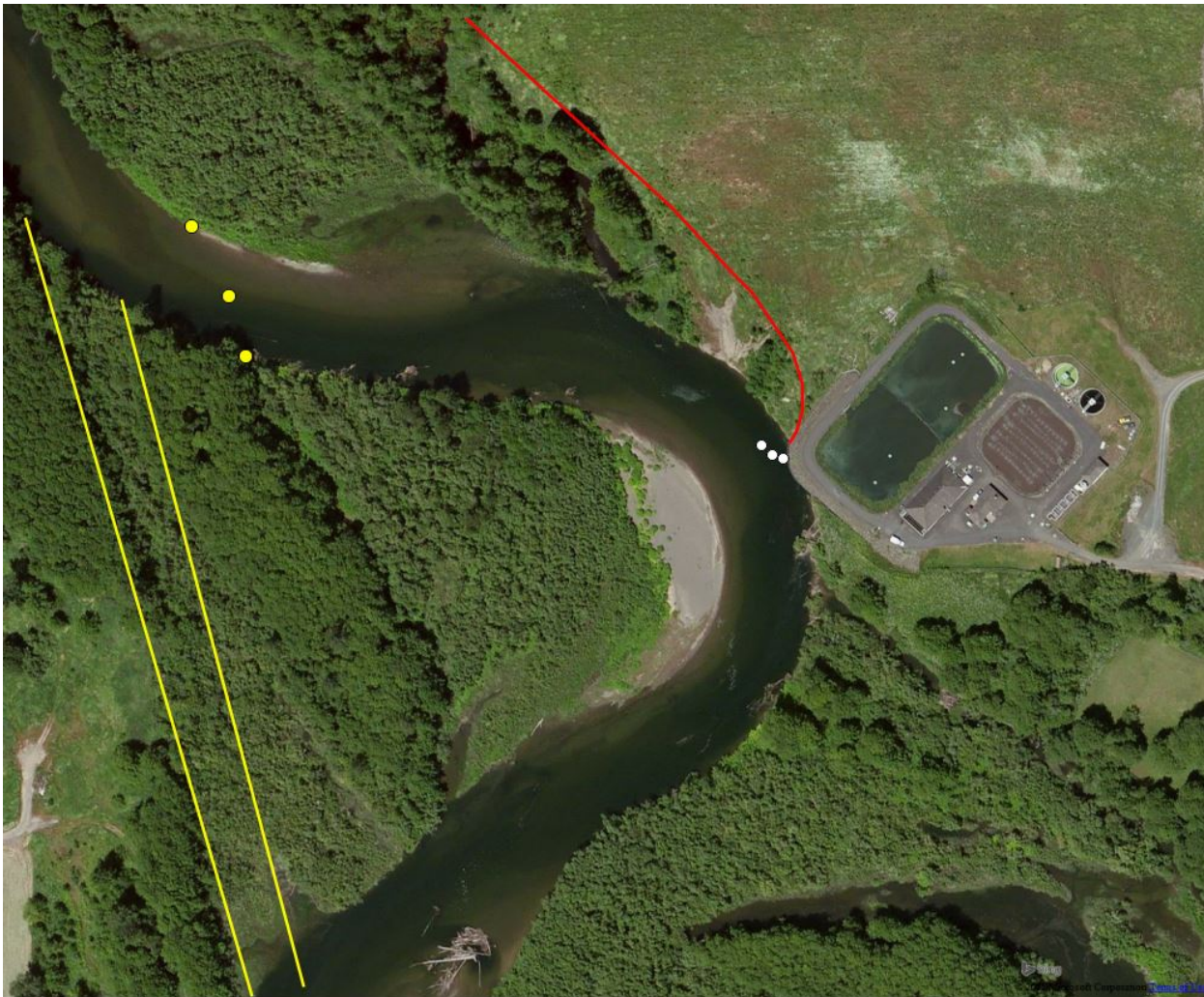
Figure 3. WWTP Vicinity with possible protection alternatives. The sheet pile wall is shown in red, while the piles are shown in the lighter color.
