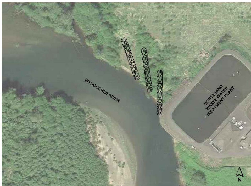
Figure 2. One alternative (Three Groin alternative) tested using the 2D model.
