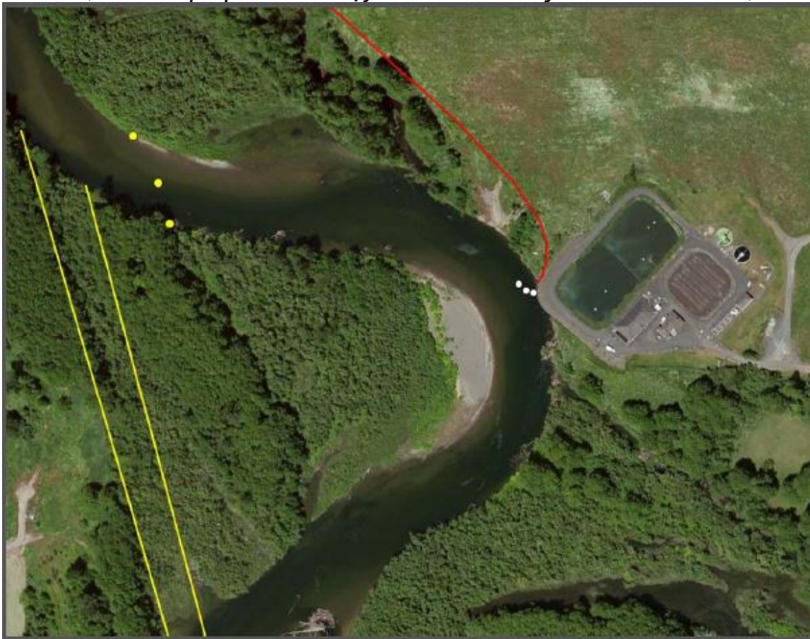
Figure 5 – Solution (red = sheet pile protection wall; yellow = redirection of river into relic channel):
