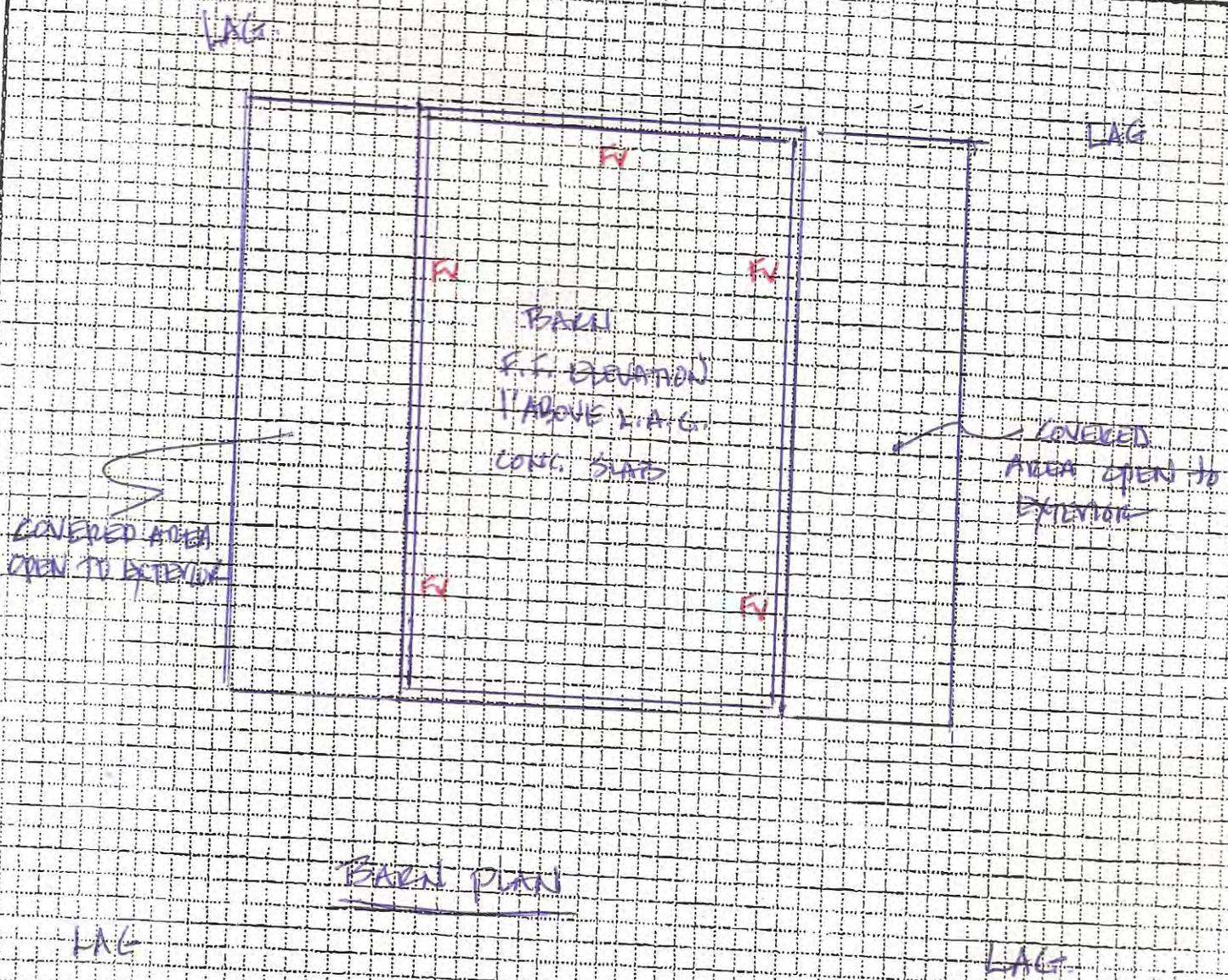
FV = SMART VENT MODEL 1540-570 (WOOD WALL)
