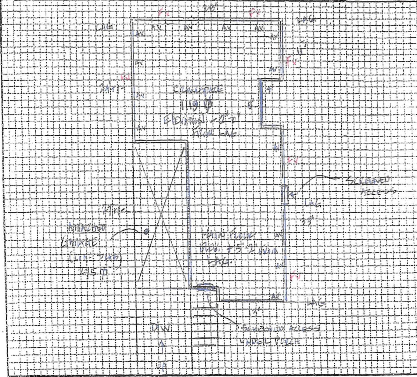
AV AIR VENTS IN TOP COURSE OF BLOCK WALL (5 COURSES ON TOP OF CONCRETE STEMWALL OF ORIGINAL FOUNDATION).
