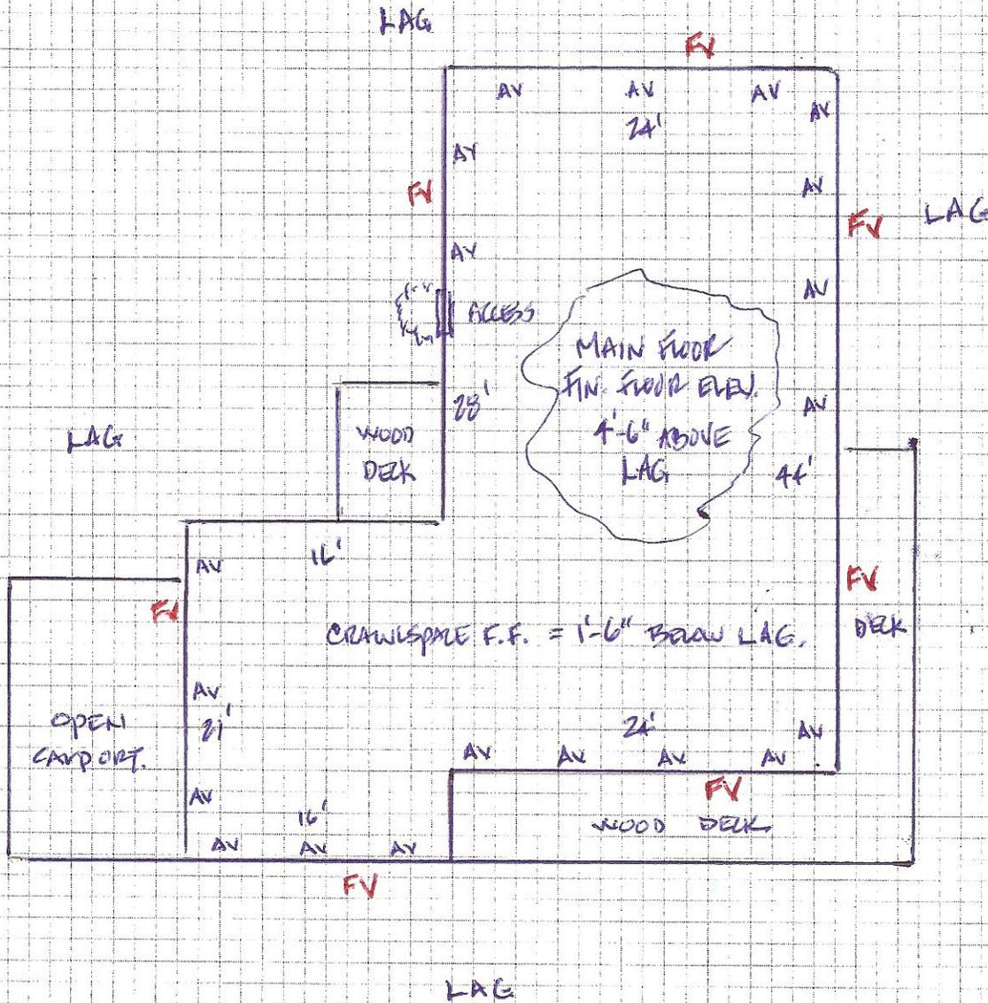
FV - SMART VENT MODEL 1540-520 INSULATED
