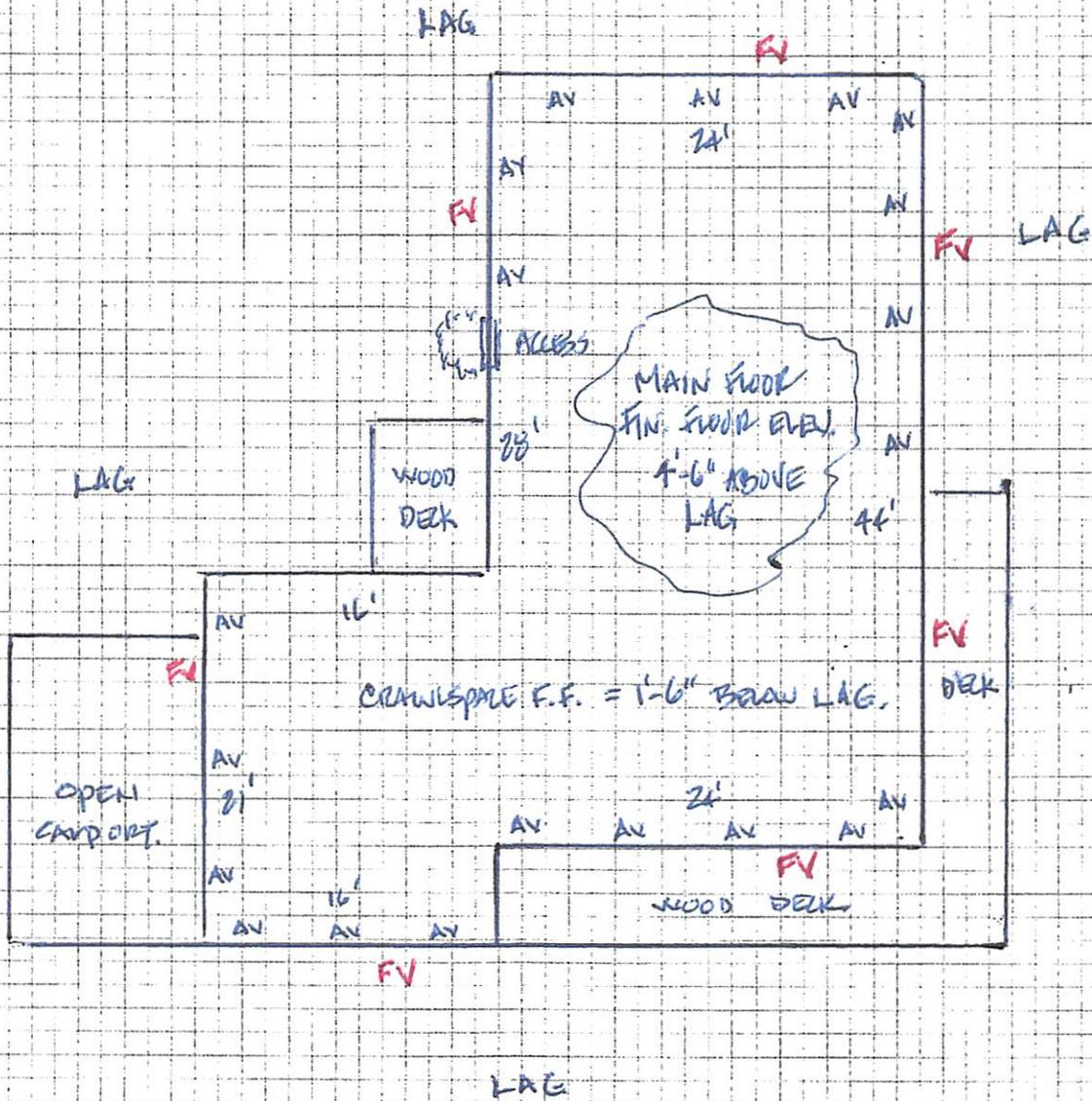
FV - SMART VENT MODEL 1540-520 INSULATED
