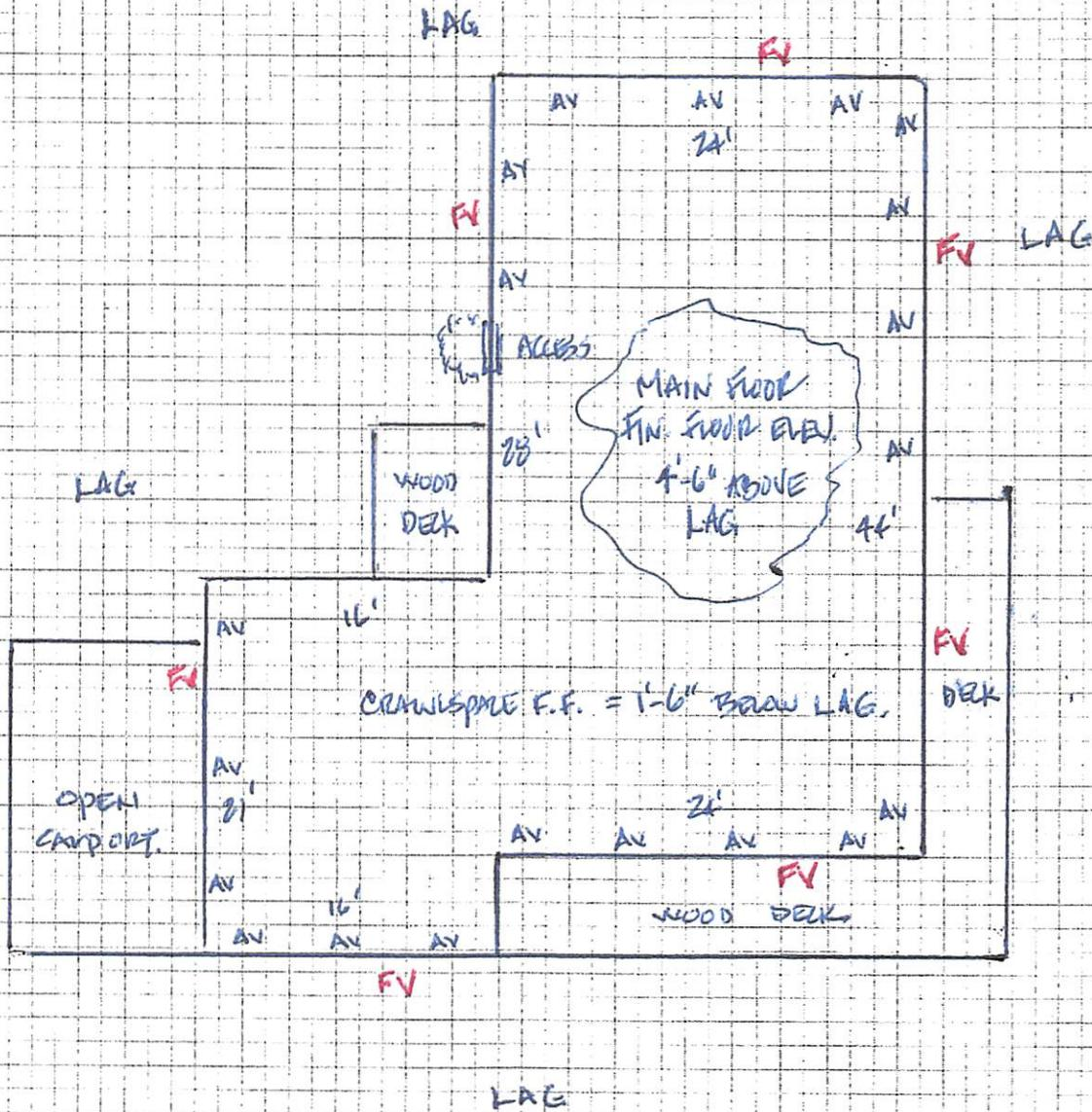
*FV - SMART VENT MODEL 1540-520 INSULATED
