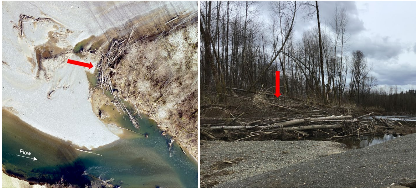
Figure 13. Example of stable log jam on the Satsop River near RM 0.5. 2019 aerial image (left) and ground-based photo (NSD, March 2019). The log jam pictured is located at the apex of the channel split between the avulsion and abandoned meander, near RM 0.5. Aerial imagery shows wood accumulation at this location as early as 2013. The majority of wood accumulation is composed of alder and cottonwood species.
