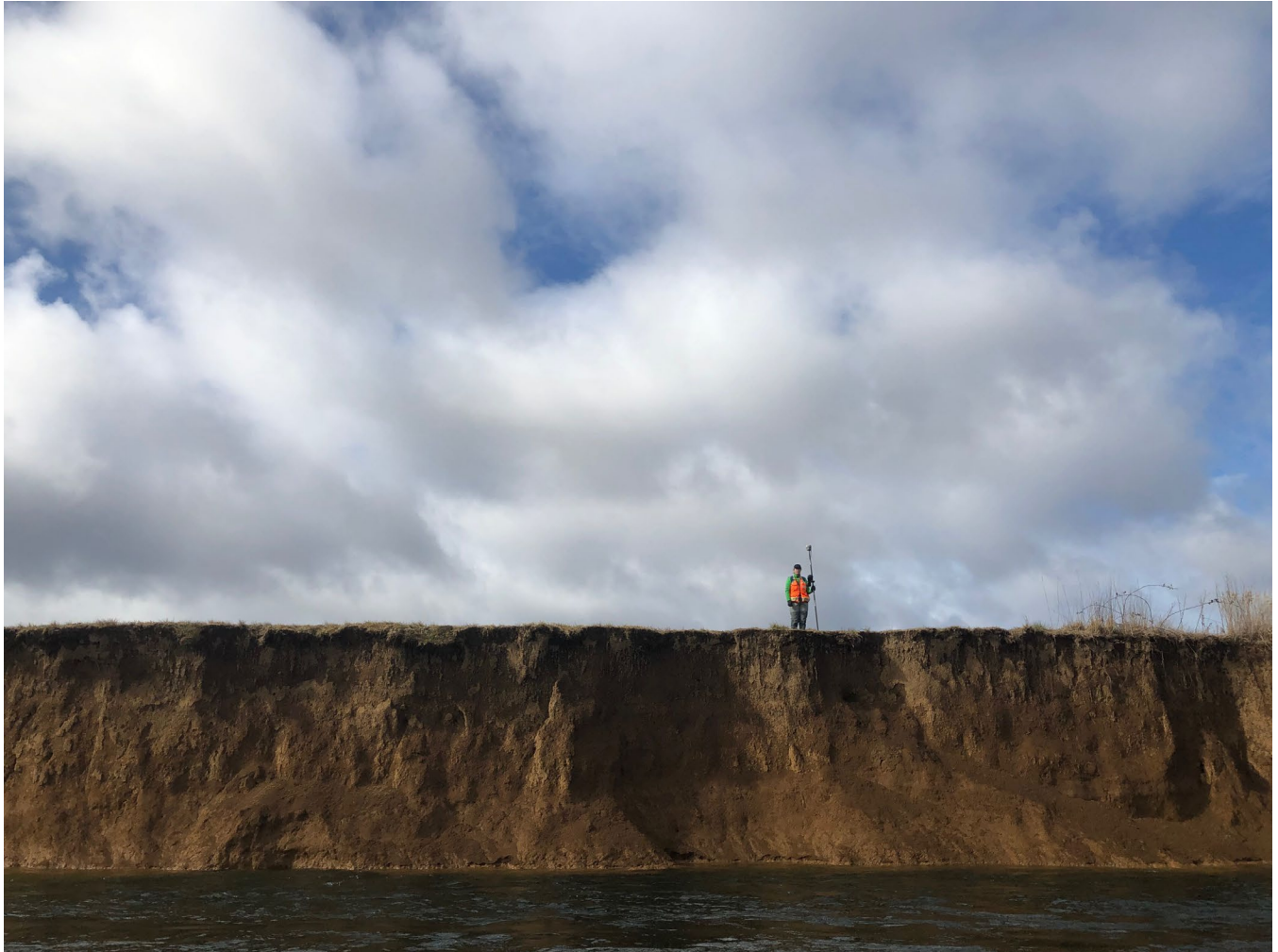
Figure 3. Eroding right bank near RM 0.2 illustrates that much of the material underlying the Satsop/Chehalis River confluence area is composed of highly erodible silts. Similar bank stratigraphic analyses were used throughout the project reach to confirm that most of the confluence area is of similar composition. Photo taken on 3/13/19.
