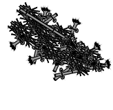
ENGINEERED LOGJAM (ELJ) TYPE 1 SETBACK REVETMENT
