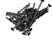
ENGINEERED LOGJAM (ELJ) TYPE 1 DEFLECTOR
