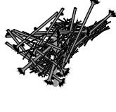
ENGINEERED LOGJAM (ELJ) TYPE 1 DEFLECTOR
