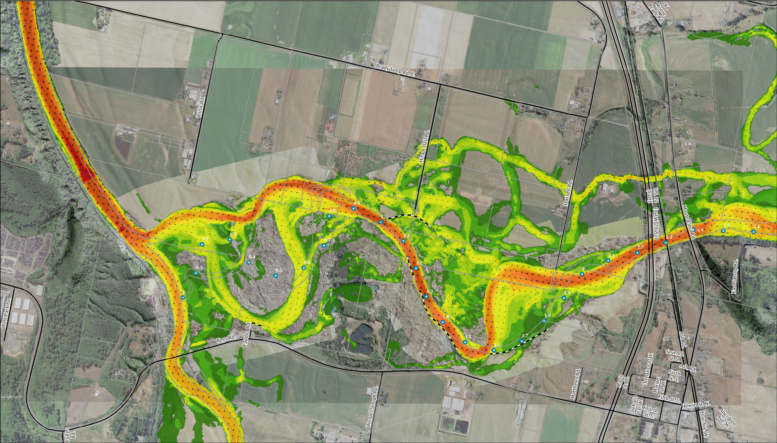
Lower Satsop River Reach Assessment and Design Proposed Conditions - Hydraulic Model Results 2-yr Flow (26,260 cfs) Velocity
