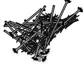
ENGINEERED LOGJAM (ELJ) TYPE 1 DEFLECTOR
