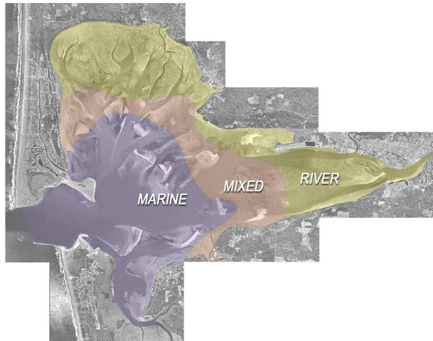
**Figure 1-2** Provinces of sand deposition in Grays Harbor as described by Scheidegger and Phipps (1976)
