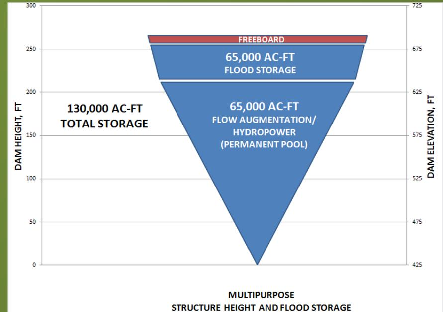
Flood Retention Crest Elevation: 654
