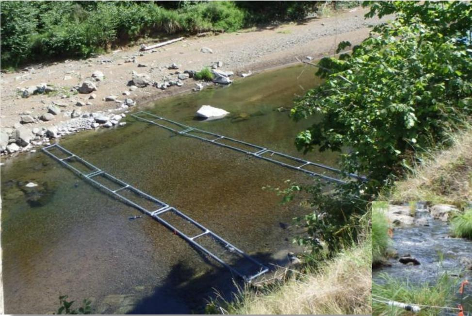
**Mainstem PIT Antenna Array near potential dam site**
