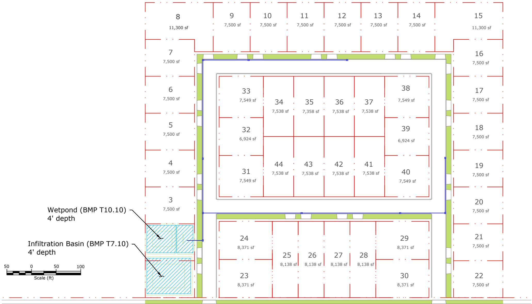
Figure 12. Scenario 1. Permanent Stormwater Site Plan – Typical Single-Family Residential Development, 2005 Requirements, Outwash Soils
