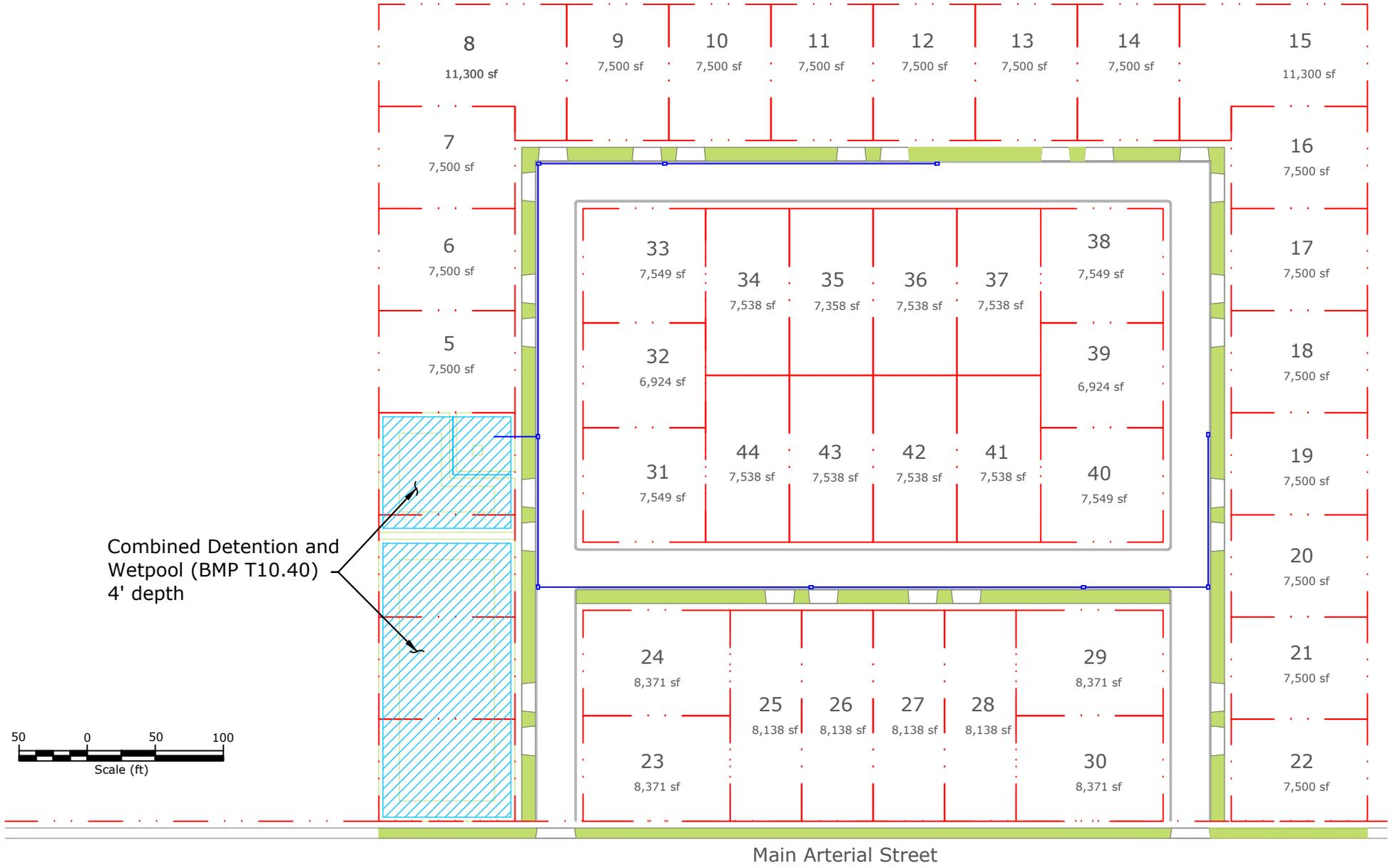
Figure 14. Scenario 2. Permanent Stormwater Site Plan – Typical Single-Family Residential Development, 2005 Requirements, Till Soils
