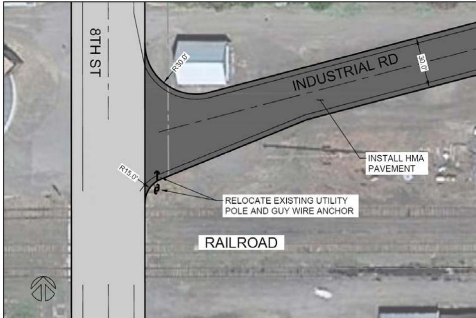
Turning path diagrams have been completed and are located in Appendix F. These diagrams show the path of the design vehicle when negotiating the intersection.
