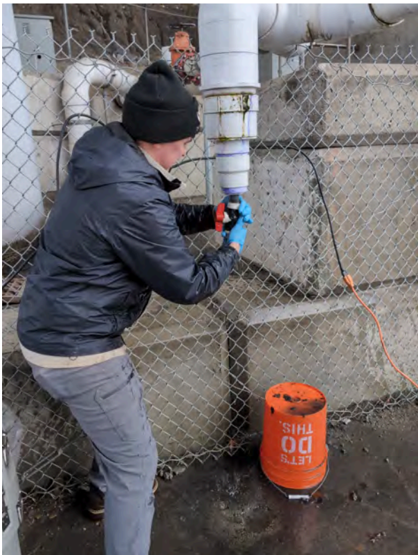
Unclogging of spigot prior to sampling (clogged with sediment build up)
