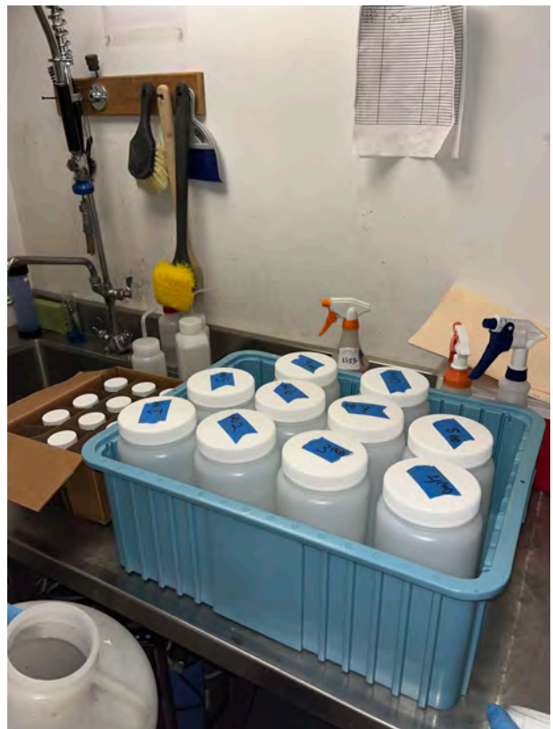
Intermediary transfer vessels (sterile, 2L HDPE) to aid transfer of 20L carboy samples to amber glass
