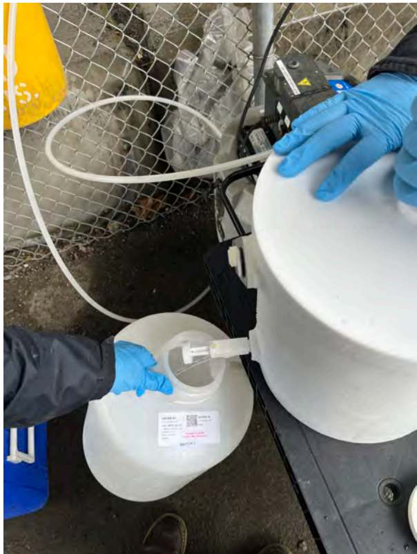
Collection of sample from churn splitter (HDPE_20L_24)
