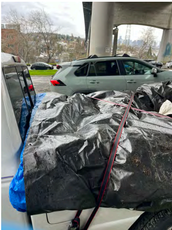
Temporary carboy preservation (ice cooled truck bed, with 2 tarps protecting carboys from direct sunlight)
