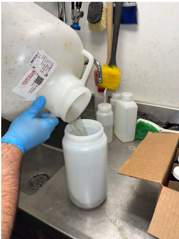
Transfer of sample from carboy to intermediary transfer vessel
