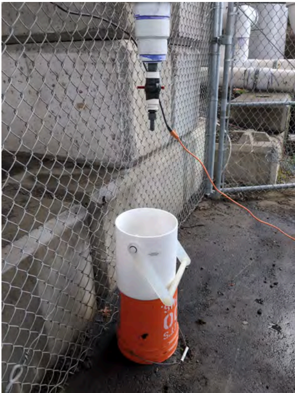
Churn splitter position for sampling
