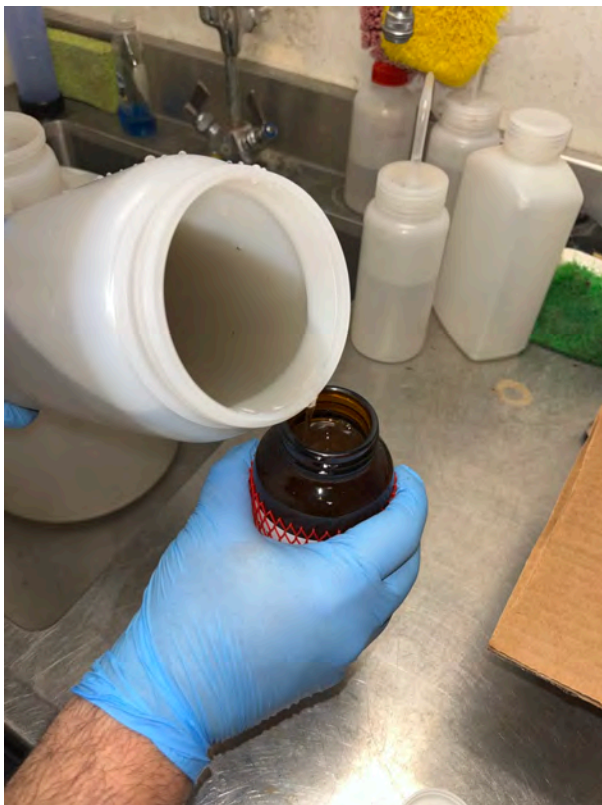
Transfer of sample from intermediary transfer vessel to amber glass bottle
