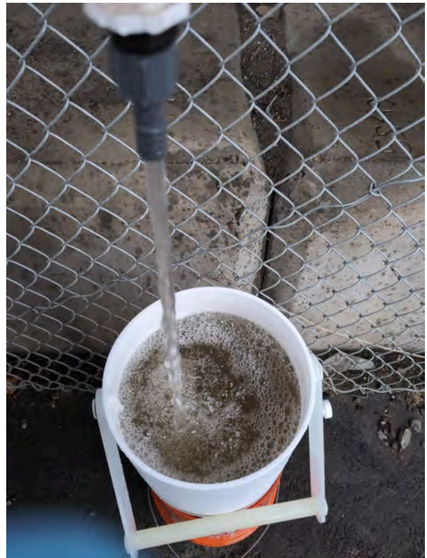
Initial rinsing of churn splitter using stormwater from sample source
