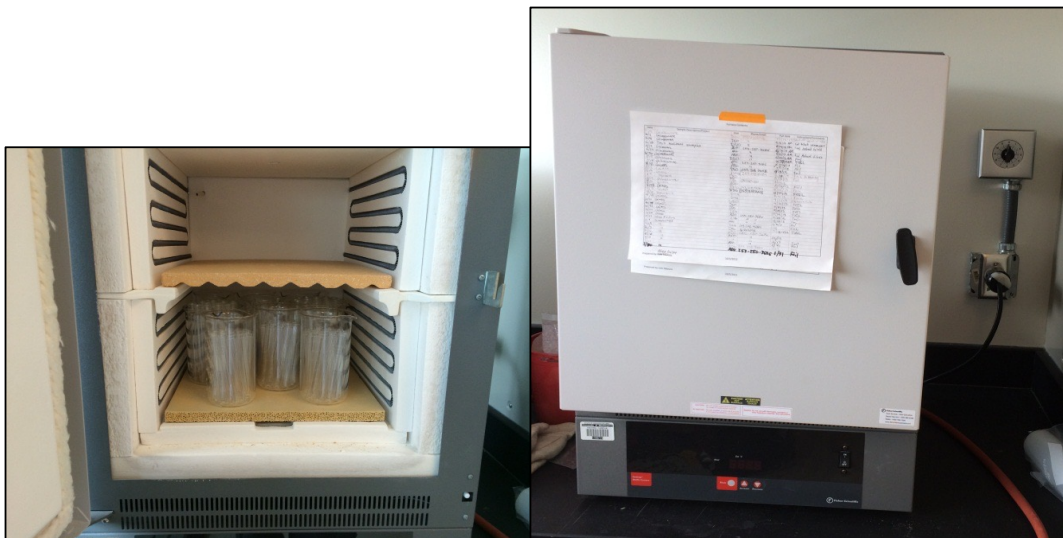
Figure 1. Glassware baking furnace. Photo on right shows control timer mounted on wall.
