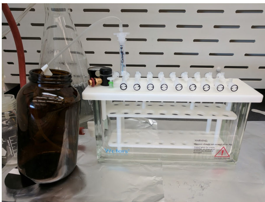
Figure 3. Extraction manifold setup during sample extraction.
