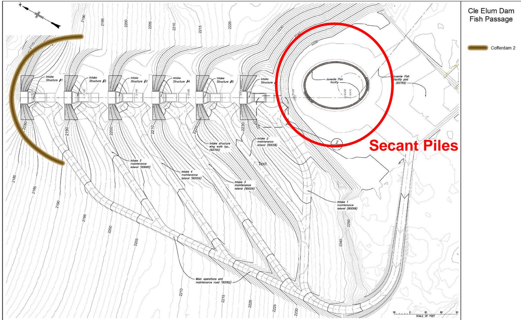
Figure 5. Juvenile Facility Intake Structure, O&M Roads, and Cofferdam #2
