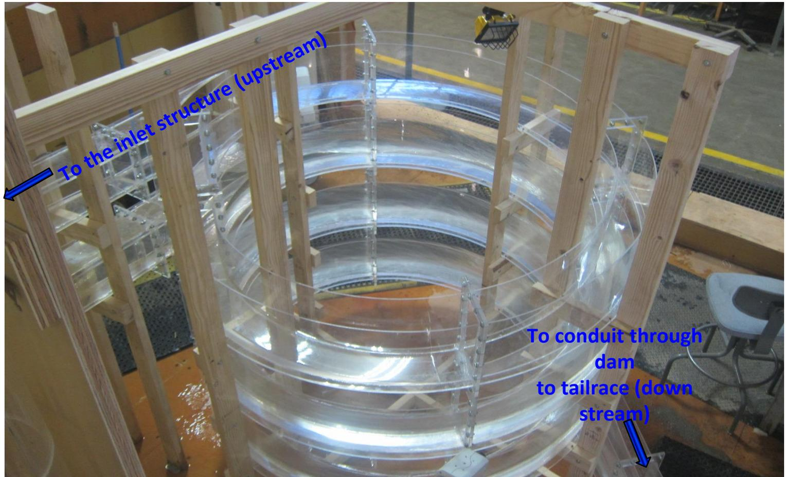
**Function – moves fish from the inlet structure into conduit bypass through the dam**
