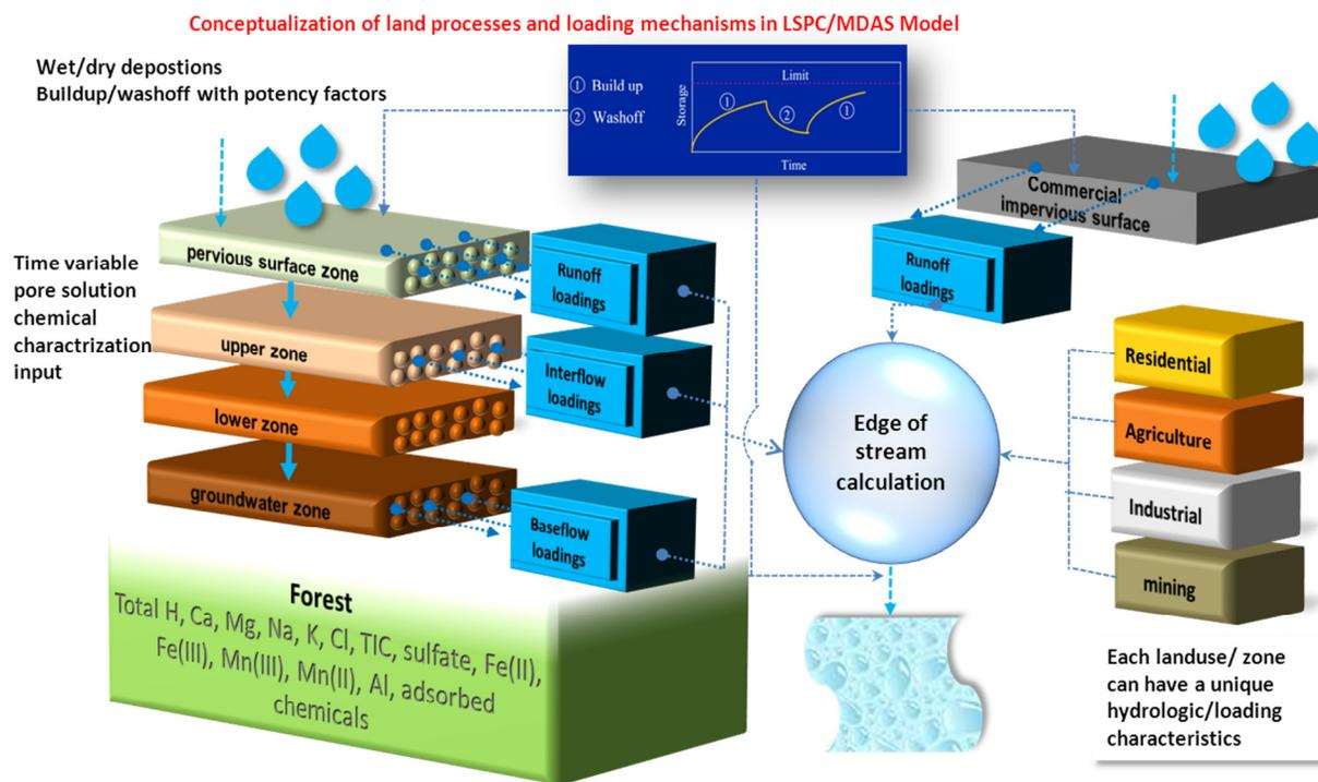
**Figure 5-4. Land components of LSPC model**
