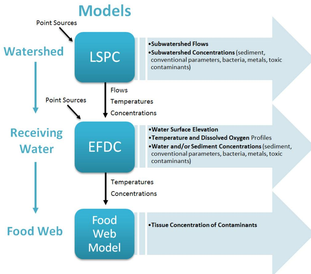
**Figure 5-2. Linked watershed-receiving water-bioaccumulation modeling framework**
