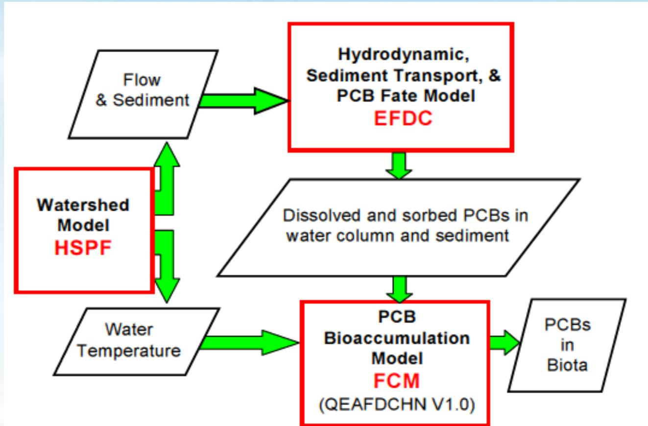
**Figure 2.** Modeling Framework for PCB Modeling of the Housatonic River Watershed.
