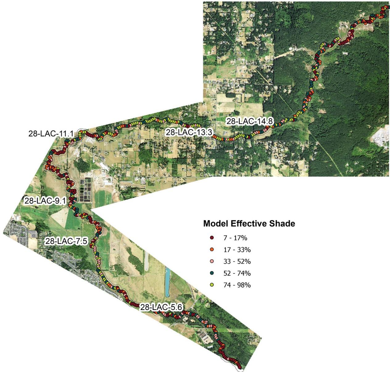
Figure 41. Model effective shade conditions for 2013 along the Lacamas Creek watershed.
