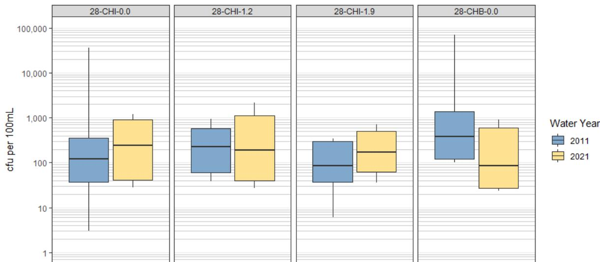
**Figure B3. Dry season fecal coliform levels for 2011 and 2021 with geometric mean (black solid line in boxplot) for sites in the China Ditch sub-watershed.**
