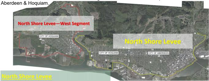
The North Shore Levee will construct a 6.2 mile levee across the two cities, providing critical flood protection and removing over 3,100 properties from FEMA's mapped Special Flood Hazard Area. The project will build resiliency in the face of future flood events, retaining existing businesses, jobs, and residents which have been on the decline in the community. The total cost of the North Shore Levee is \$78 million and is divided in four phases.
