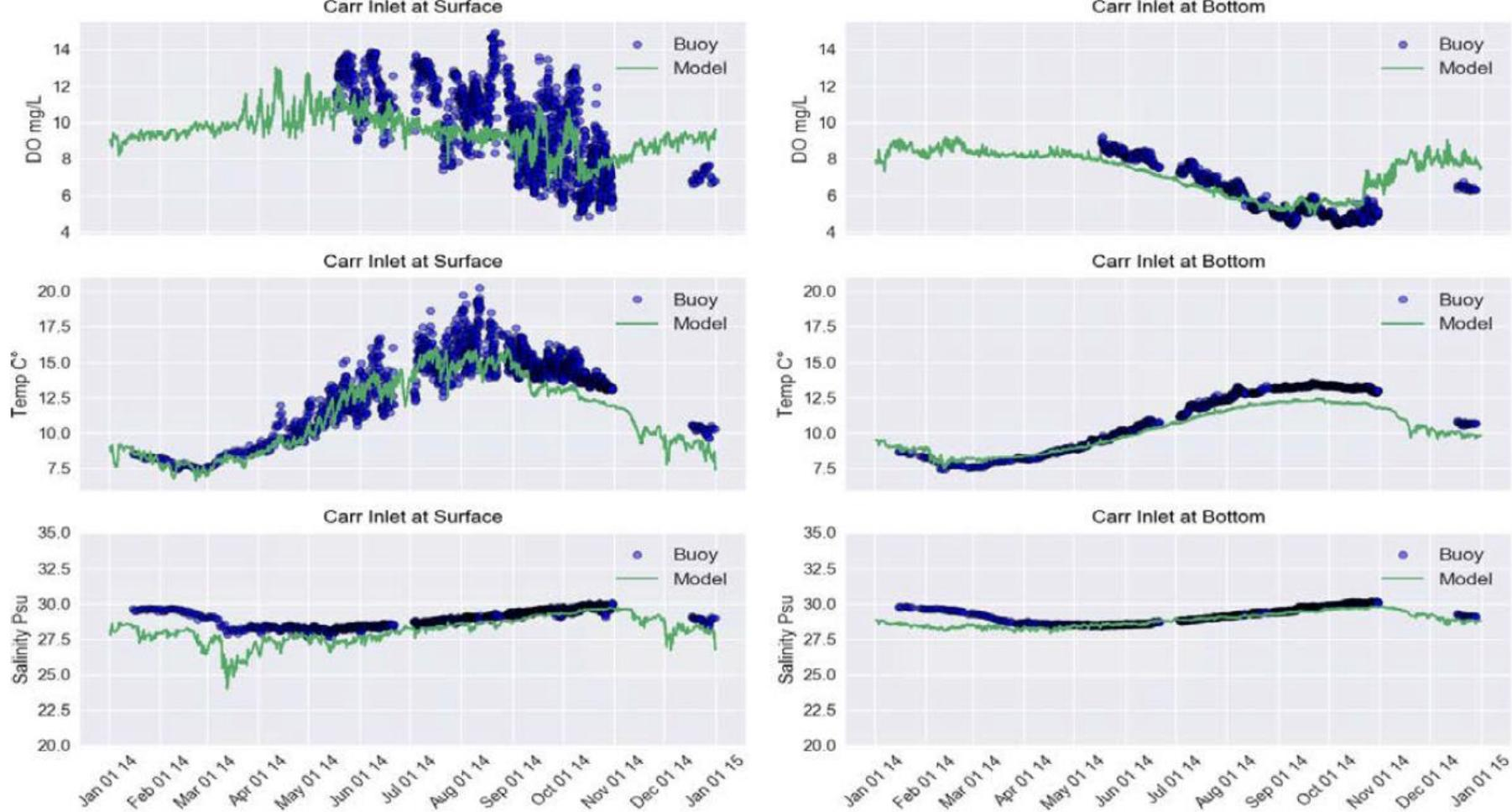
Figure J6: 2014 SSM vs. Carr Inlet buoy data for DO, temperature, and salinity at surface and bottom layers. Model results are captured at a 1 hour frequency while ORCA data collection frequency largely varies.
