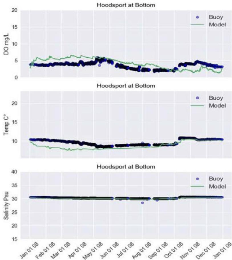
Figure J4: 2008 SSM vs. Twanoh buoy data for DO, temperature, and salinity at surface and bottom layers. Model results are captured at a 1 hour frequency while ORCA data collection frequency largely varies.
