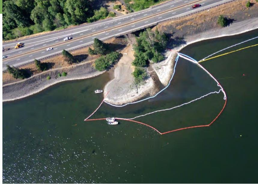
Containment of a discharge from an outfall
