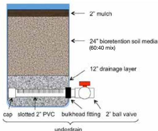
Diagram of bioretention unit using 55-gallon drum.
