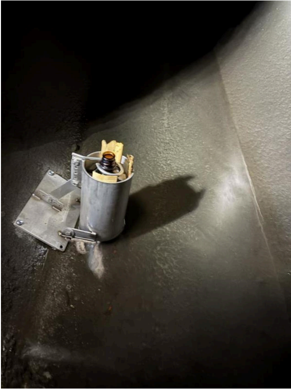
close-up view of one sediment trap installed within the pipe
