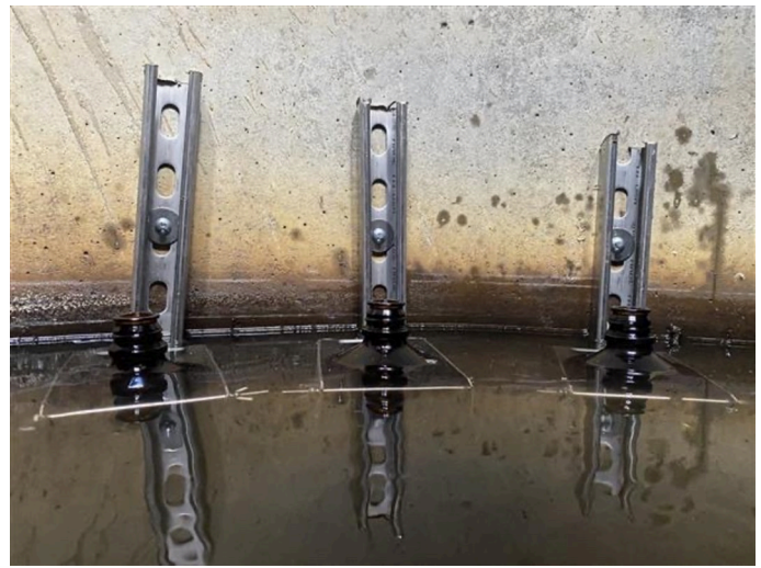
Close-up view of sediment traps
