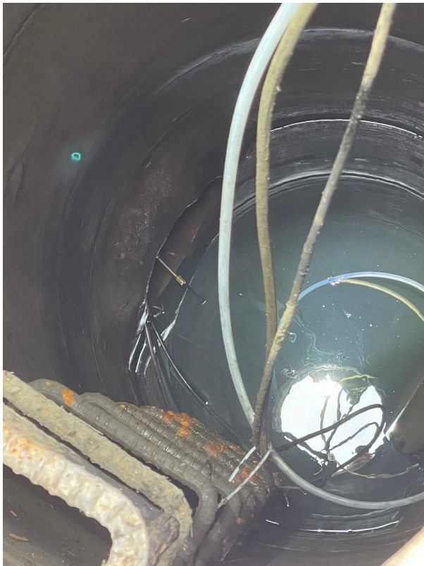
Intake tubing for autosampler goes directly into the sump.
