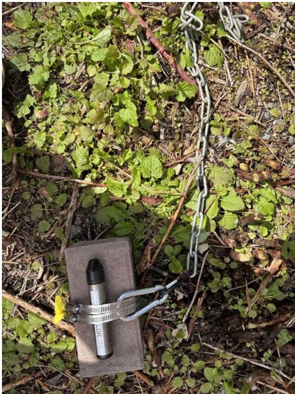
Photo of pressure transducer setup before installation (hose clamped to a brick, which a chain for attachment).
