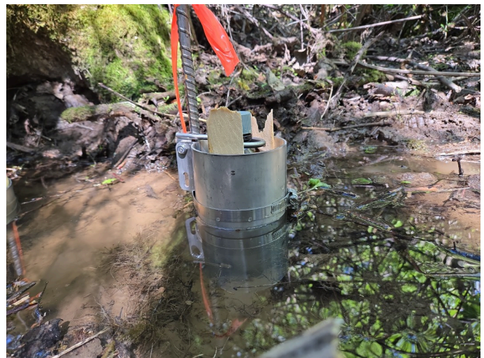
close-up view of sediment trap (side view)
