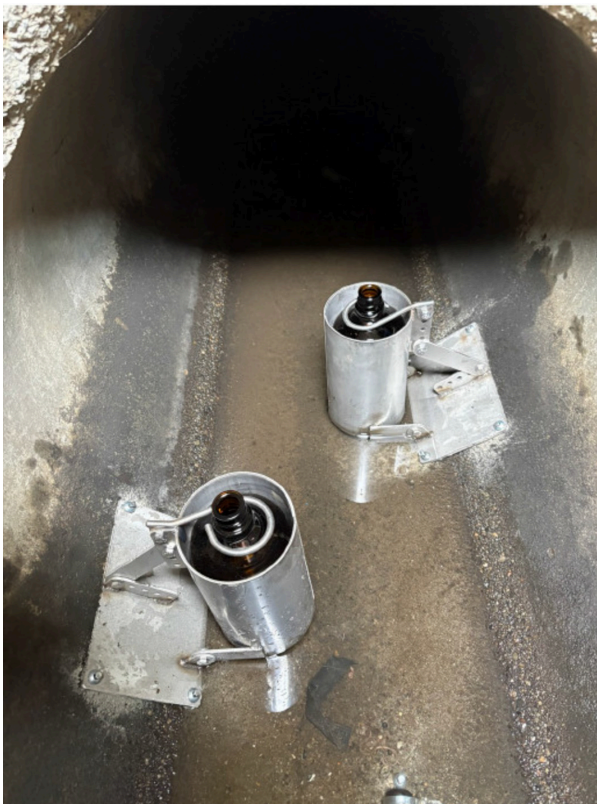
Two of three sediment sampler locations
