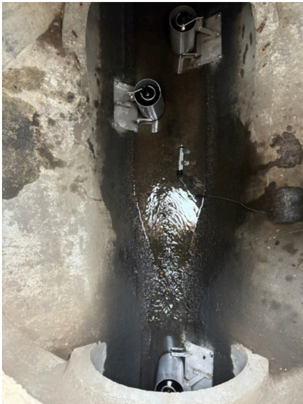
Bird's eye view of all three traps and pressure transducer
