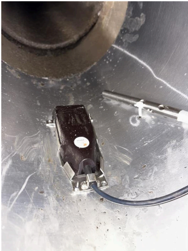
Close-up of Sampler intake tubing in relation to flow sensor.
