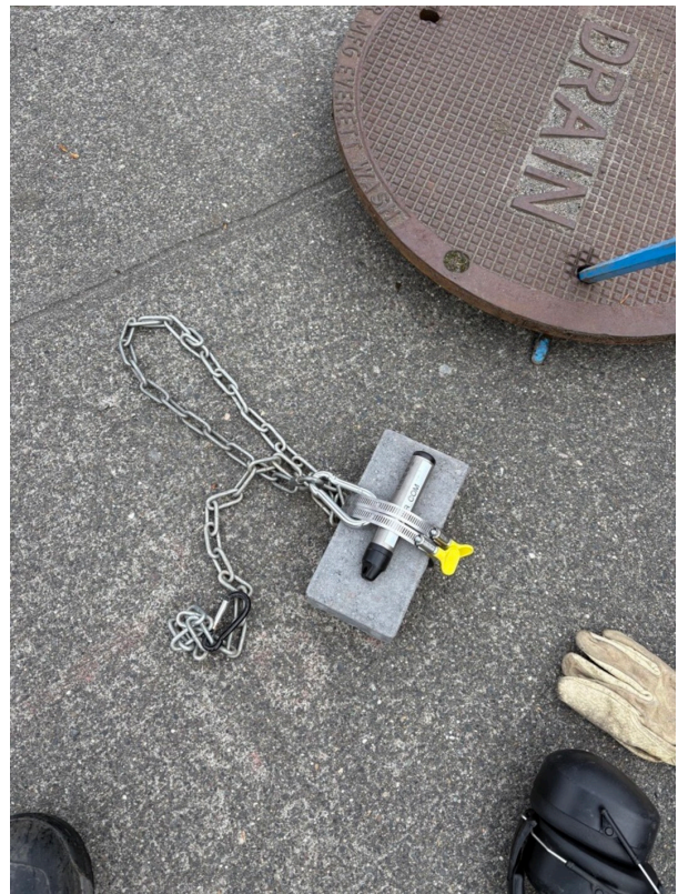
Photo of TROLL prior to installation. The TROLL is hose clamped to brick with a chain attachment.
