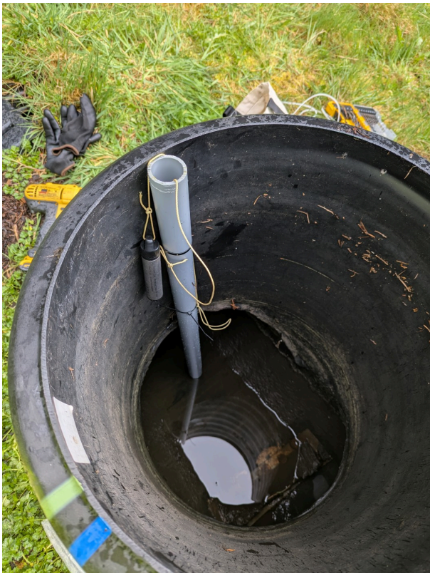
Location of barro TROLL and level TROLL inside conduit pipe.
