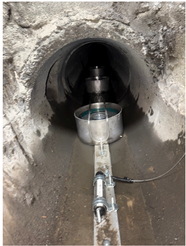
Sediment traps inside pipe
