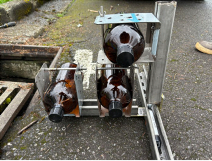
Pressure Transducer location on trap mount before installation.
