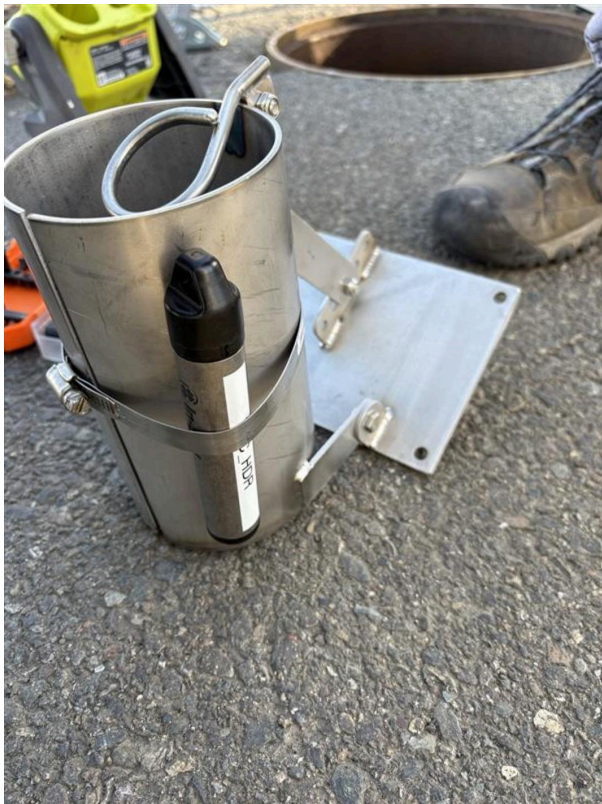
Location of pressure transducer on sediment trap before installation
