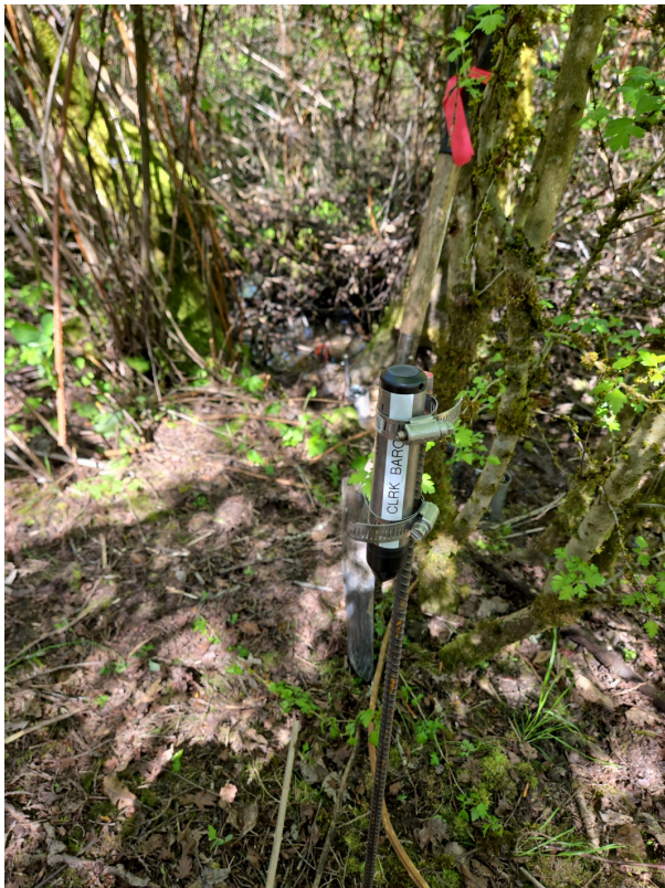
Pressure Transducer set up before installation in stream
