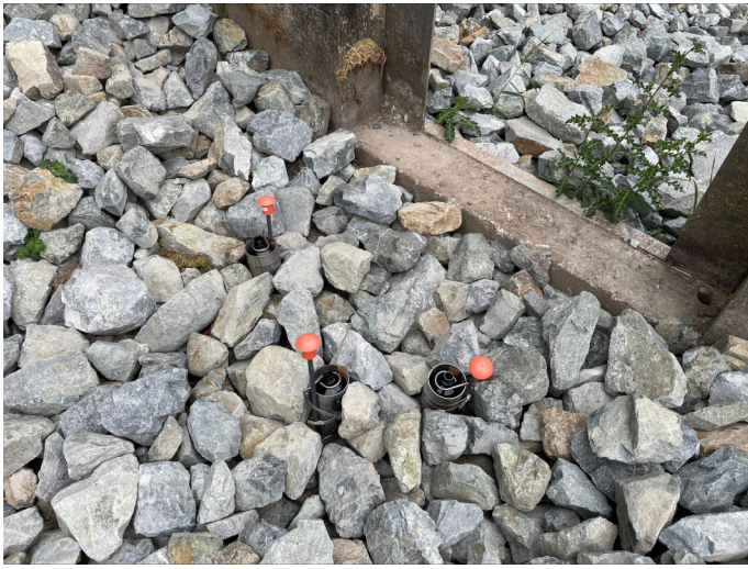
top view of the three sediment traps.
