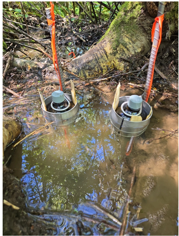
close-up view of sediment trap (bird-eye view)
