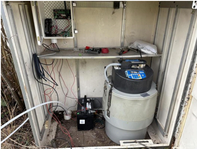
Enclosure showing the ISCO autosampler, Campbell datalogger and power system. View of tubing going into pipe system
