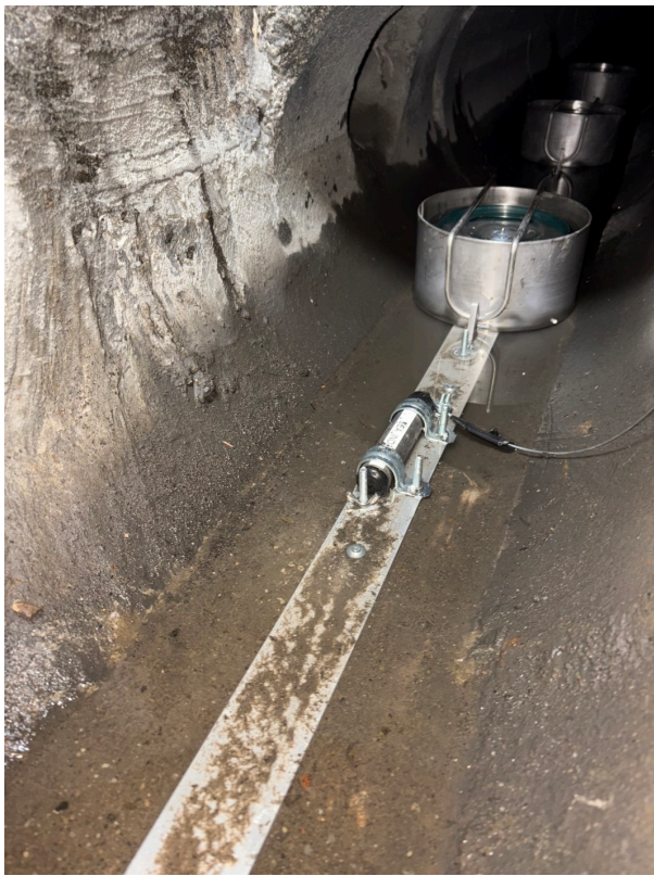
Location of Pressure transducer in relation to sediment traps
