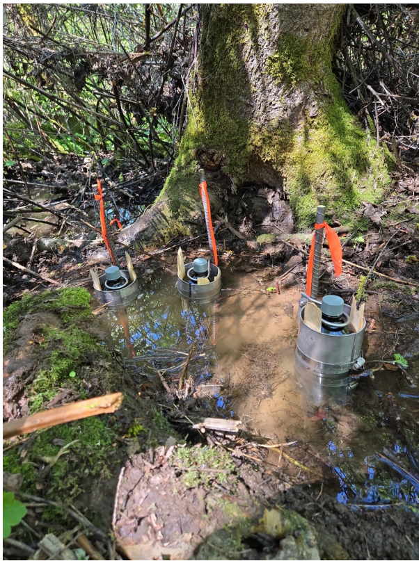
Location of sediment traps inside channel
