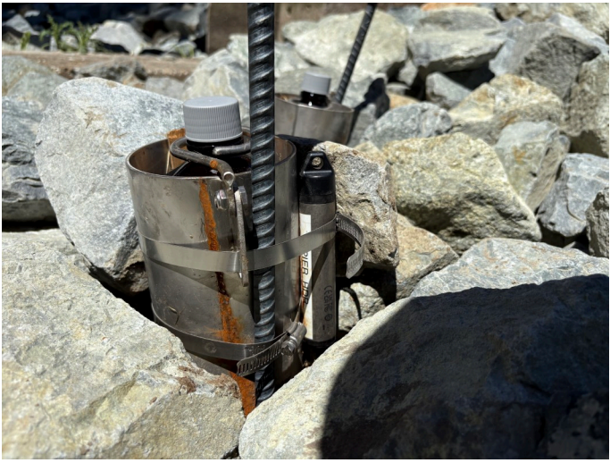
Pressure transducer hose clamped to one of the sediment traps.
