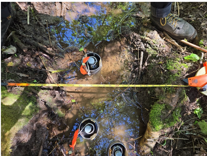
Width of channel where traps are installed. Shows that stream width is about 1.5ft
