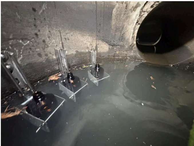
Sediment trap locations inside the CB
