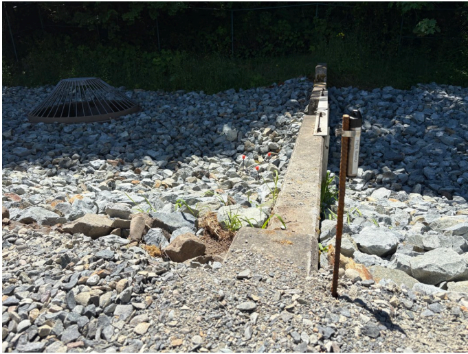
Barometric sensor hose clamped to rebar pipe which is pounded into the ground next to the concrete weir wall.
