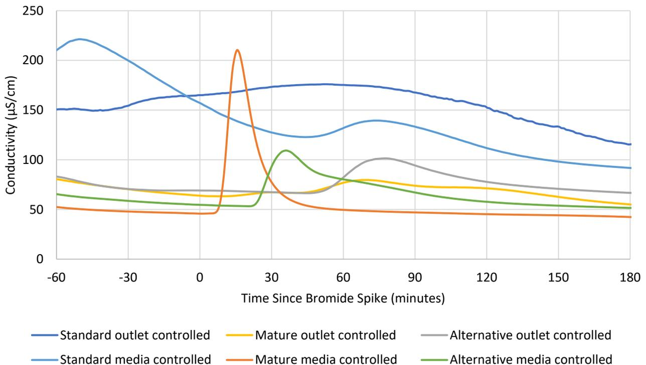
Figure 1. Hydraulic residence time testing results
