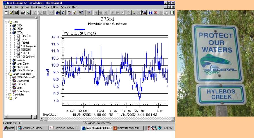
*Example of Flow Link software data file for S. 373<sup>rd</sup> Street – Dissolved Oxygen 9/10/02-11/10/02*
