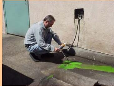
*Bright-colored dyes are used to track stormwater flows*
