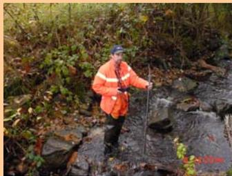
*SWM staff calculating total stream discharge in West Hylebos Creek using a hand-held current velocity meter*
