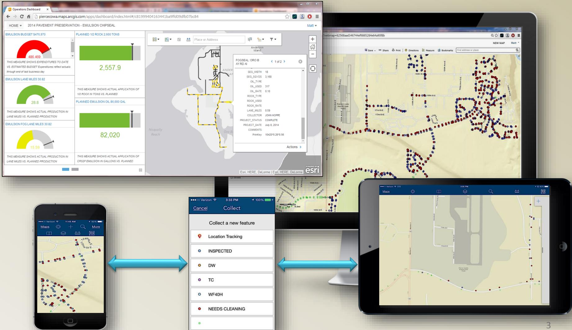
The image illustrates a multi-device asset management system. At the top left is a desktop browser window showing an 'Operations Dashboard' for '2014 PAVEMENT PRESERVATION - EMULSION CHIPSEAL'. The dashboard includes several gauges and bar charts:
