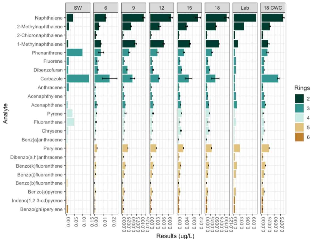
**Figure A1.1.** PAH concentrations in influent clean water (Lab), influent stormwater (SW), and triplicate samples of effluent from each of the five treatment depths (6", 9", 12", 15", 18") plus the clean water control (18" CWC) during Event 1. Error bars are one standard error of the mean. One-half of the value of the detection limit (DL) was substituted for the value of non-detects.
