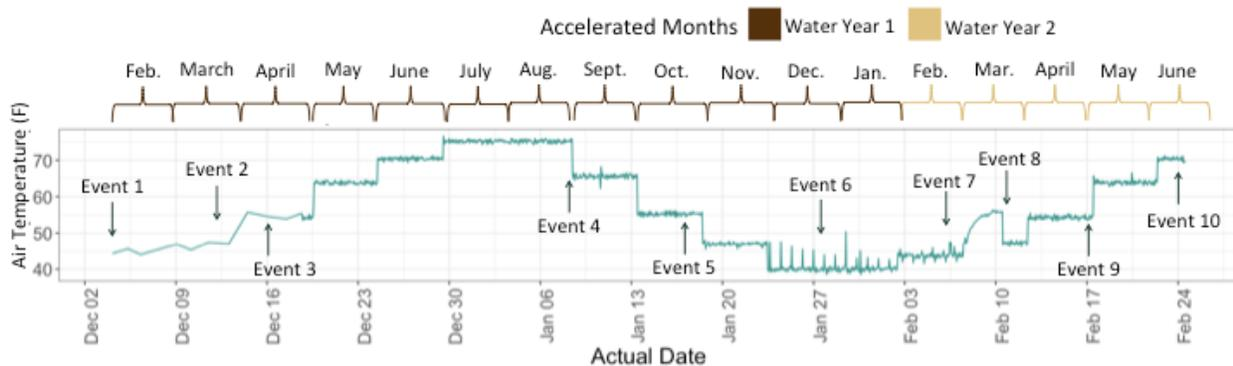
**Figure 4.** Timeline of temperatures (F) in the environmental chamber during the first 10 events.
