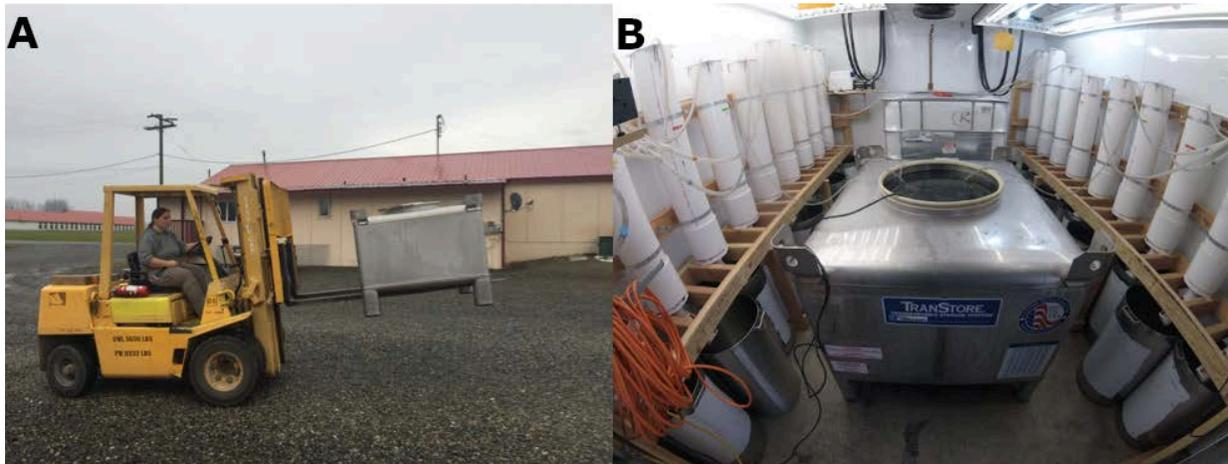
**Figure 3.** A) Transportation tanks filled with stormwater runoff are moved into the temperature-controlled chamber. B) The clean water tank (rear) and stormwater transportation tank (front) in the temperature-controlled chamber with the experimental columns.
