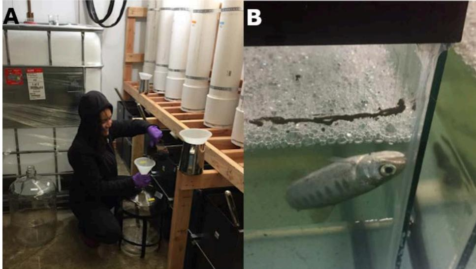
**Figure 7.** A) Effluent from the bioretention columns to be used for toxicity testing using juvenile coho salmon is collected into glass carboys. B) Juvenile coho salmon exposed to 100% urban stormwater runoff suffering from loss of equilibrium.
