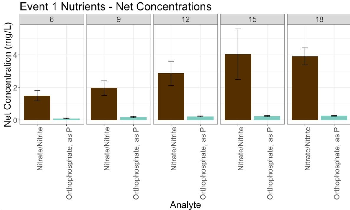
**Figure 6.** Mean (standard error) net concentration (effluent minus influent) for nutrients among the five treatment depths.
