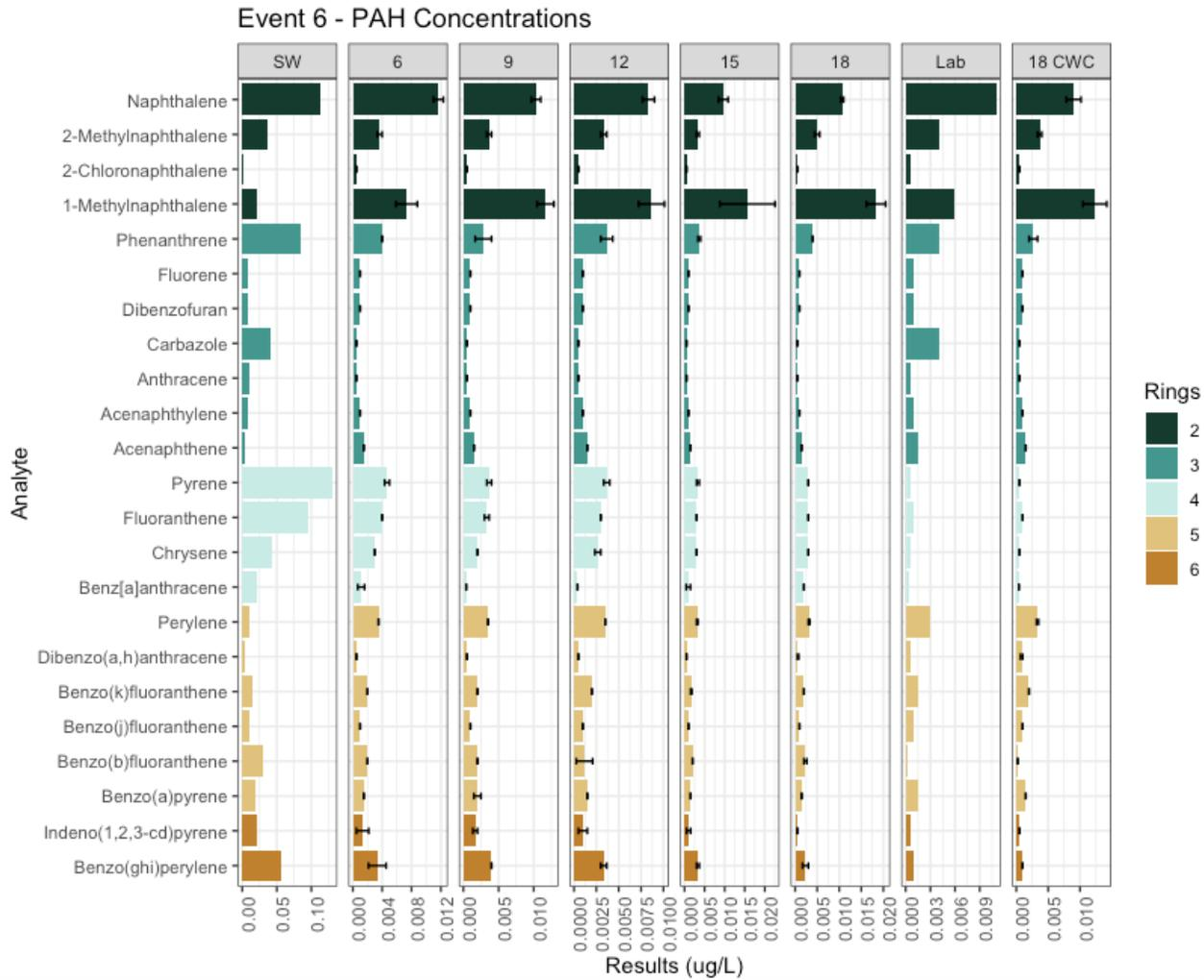
**Figure A1.2.** PAH concentrations in influent clean water (Lab), influent stormwater (SW), and triplicate samples of effluent from each of the five treatment depths (6", 9", 12", 15", 18") plus the clean water control (18" CWC) during Event 6. Error bars are one standard error of the means. One-half of the value of the detection limit (DL) was substituted for the value of non-detects.
