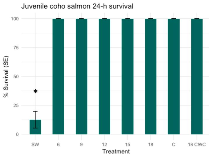
**Figure 8.** Survival of juvenile coho salmon following 24-h exposure to urban stormwater runoff influent (SW) and bioretention-treated runoff pooled across triplicates of each bioretention treatment depth (6", 9", 12", 15", 18", and 18" clean water control (CWC)). An asterisk indicates that an exposure significantly affected survival relative to controls.
