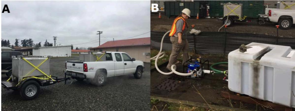
**Figure 2.** A) Stainless steel transportation tanks at the WSU-Puyallup campus ready to transfer stormwater from the collection site. B) Stormwater runoff pumped from the polyethylene collection tanks to the stainless steel transportation tanks using a gas-powered pump and food-grade hosing.
