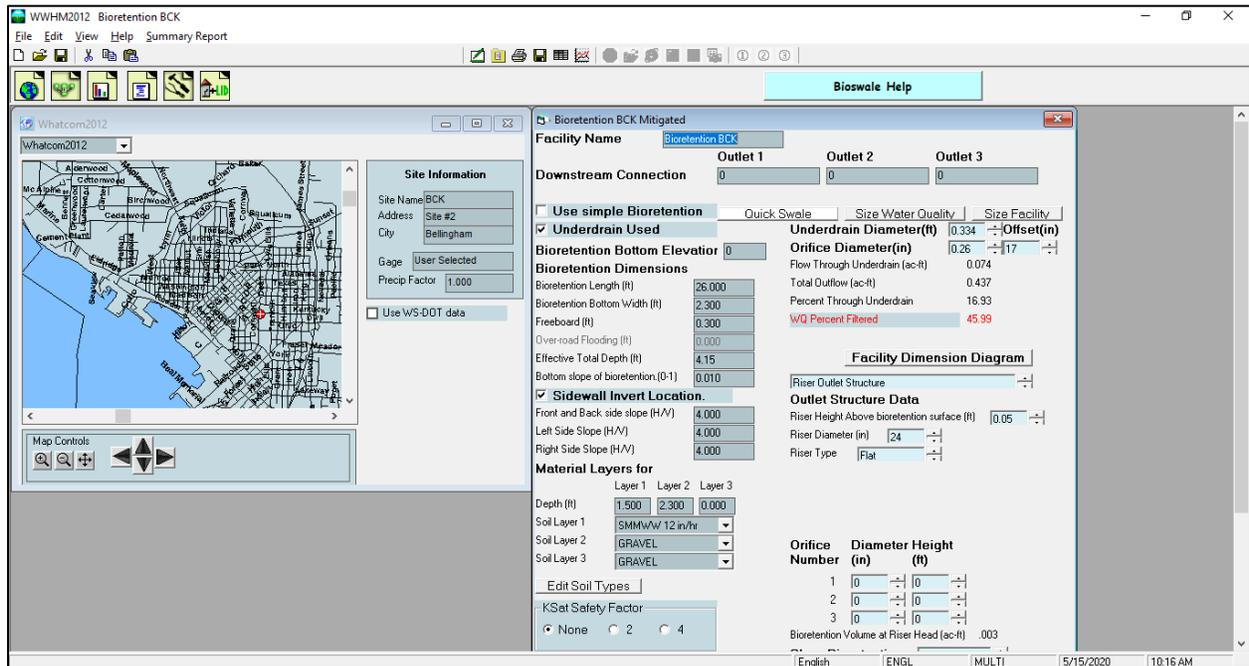
The BCK bioretention site is located in Bellingham, Whatcom County, Washington. The drainage area to BCK consists of 0.27 acres of roads on a flat slope (0-5%).
