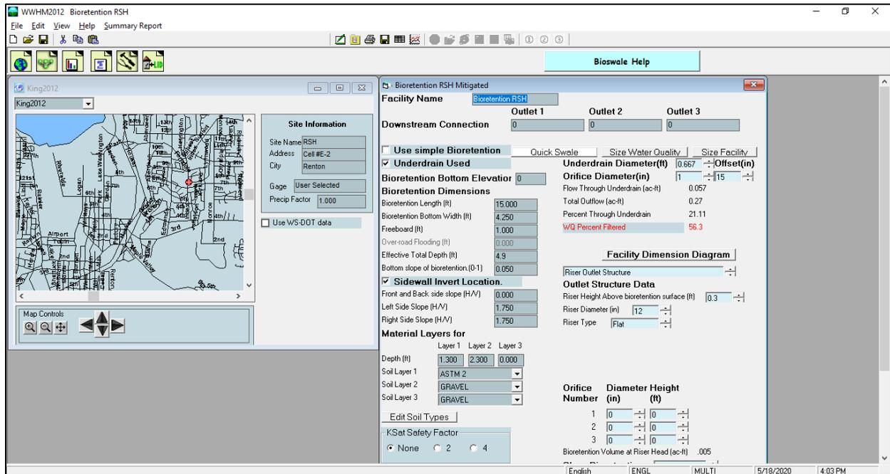
The RSH bioretention site is located in Renton, King County, Washington. The drainage area to RSH consists of 0.0283 acres of A/B soil, lawn vegetation, on a moderate slope (5-15%), and 0.1417 acres of roads on a moderate slope (5-15%).
