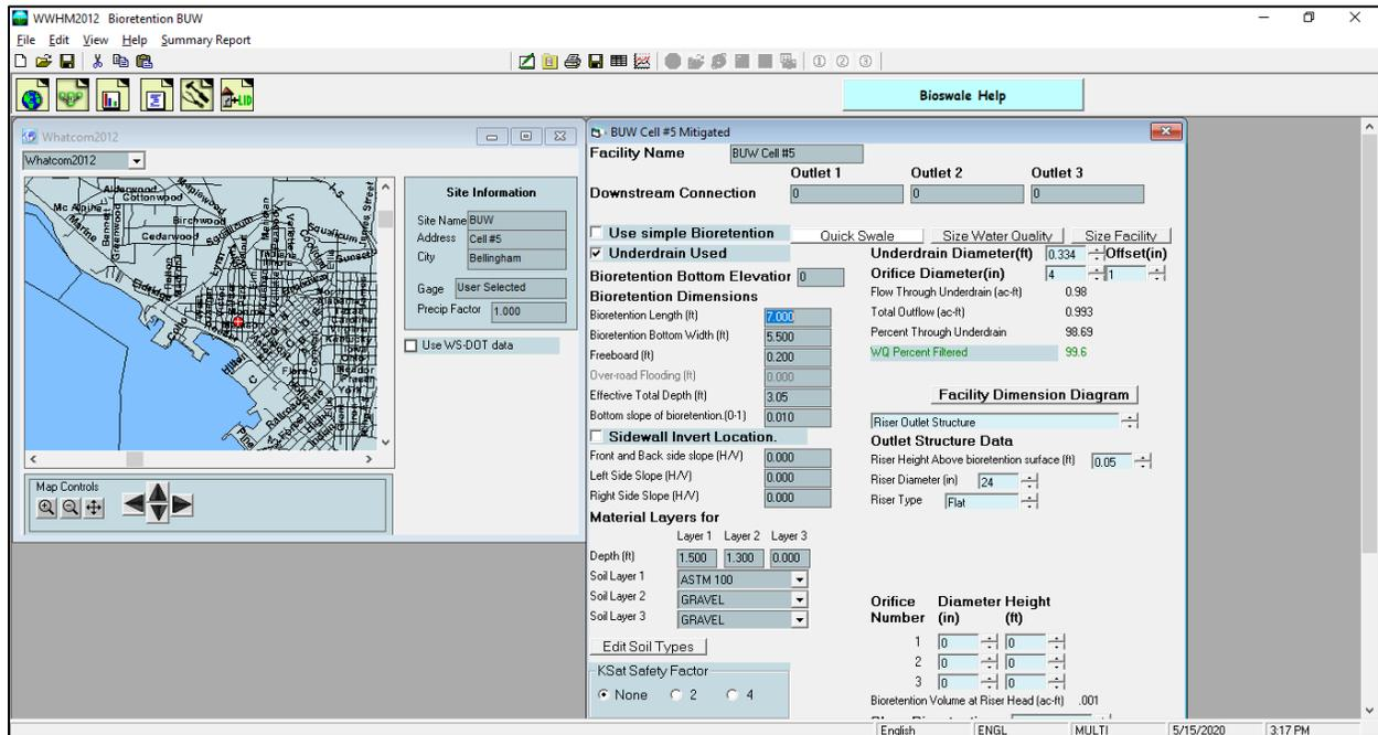
The BUW bioretention site is located in Bellingham, Whatcom County, Washington. The drainage area to BUW is a neighborhood consisting of 0.49 acres of C soil, lawn vegetation, on a flat slope (0-5%), 0.26 acres of roof, and 0.18 acres of road on a flat slope.
