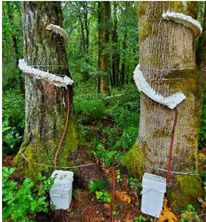
*Figure 8: Stem flow buckets placed beneath stem flow collars on a Douglas-fir (left) and bigleaf maple (right) at the Evergreen Organic Farm (plot 2).*
