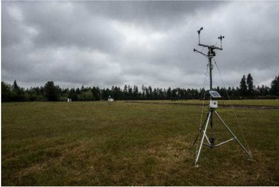
Figure 6: Weather station placed in a field north of the Webster plots. Additional nearby weather stations used by AgWeatherNet were used for data quality assurance.
