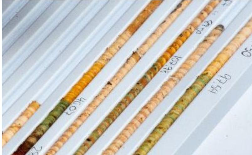
Figure A17: Bromocresol green stained sapwood in several Douglas-fir core samples.
