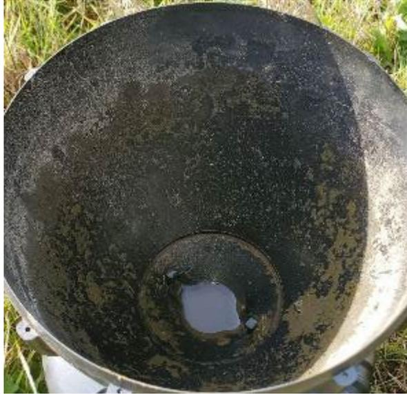
*Figure A15: A rain gauge clogged with dirt and pollen which was able to penetrate the protective mesh covering.*
