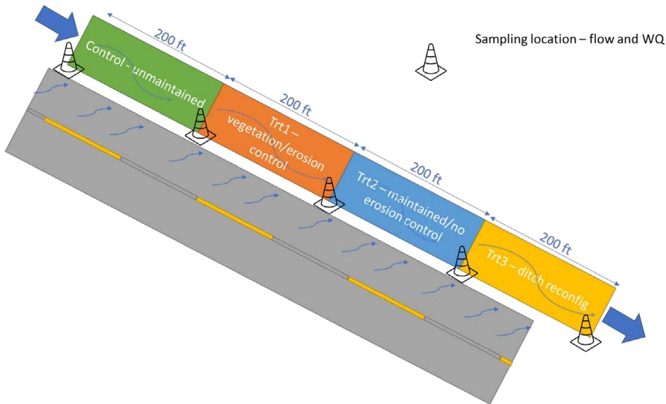
Figure 1: Arrangement of control and three treatment sections for this study.
