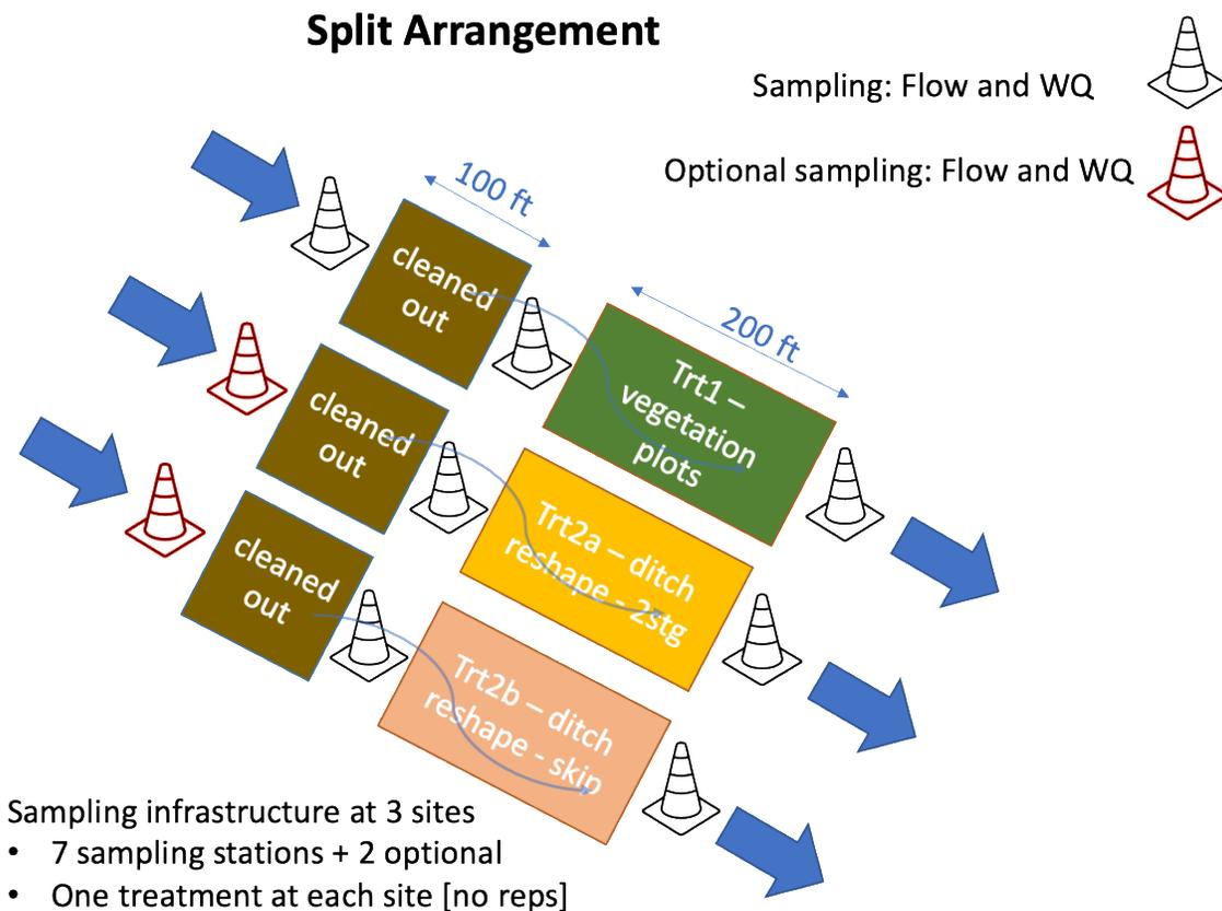
Figure 1: Split arrangement of three alternate vegetation and retrofit experimental setups. One of each experimental setup will be implemented at a site – with three sites total. Arrows denote flow direction.
