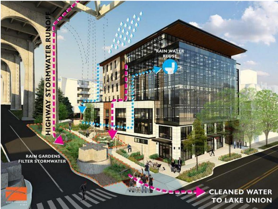
**Figure 4:** Schematic Illustration (top) and Construction Document excerpt (bottom) of Bioretention Design for Phase III, under construction Spring 2020. Proposed full monitoring of stormwater and soils.
