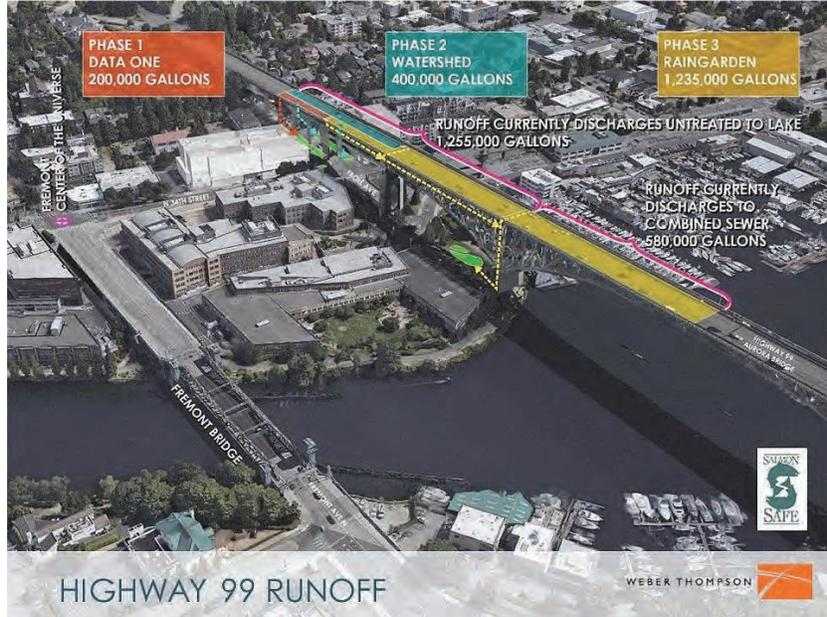
**Figure 2.** Stormwater Runoff-Producing Drainage Basins and Storm Drain System (left), and Location and Concept Design of Aurora Bridge Phase III Bioretention Unit (right)
