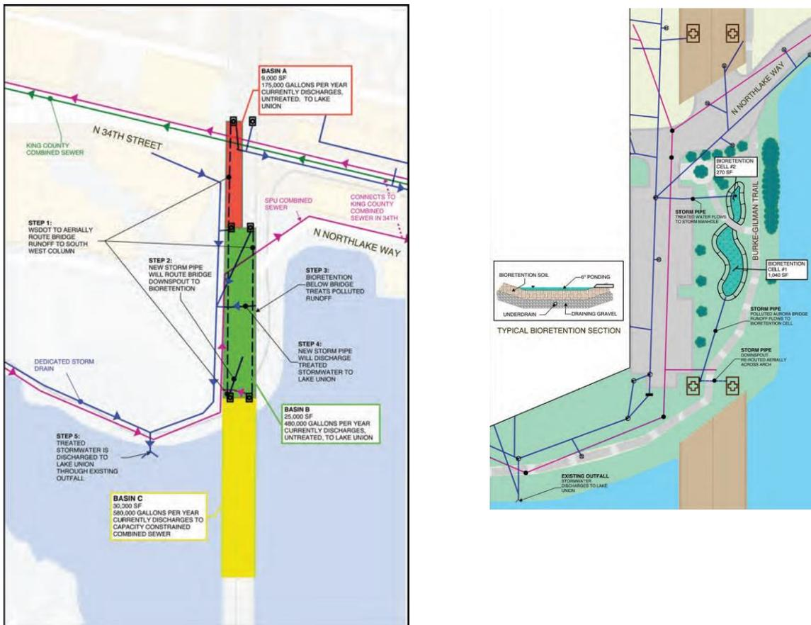
**Figure 3.** Aurora Bridge Bioretention Phases I and II, Completed (top) and Under Construction (bottom). Proposed grab sample monitoring.
