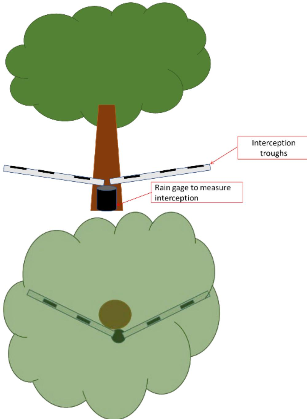
Figure 6: Profile (top) and plan (bottom) views of troughs and rain gage used to measure canopy throughfall
