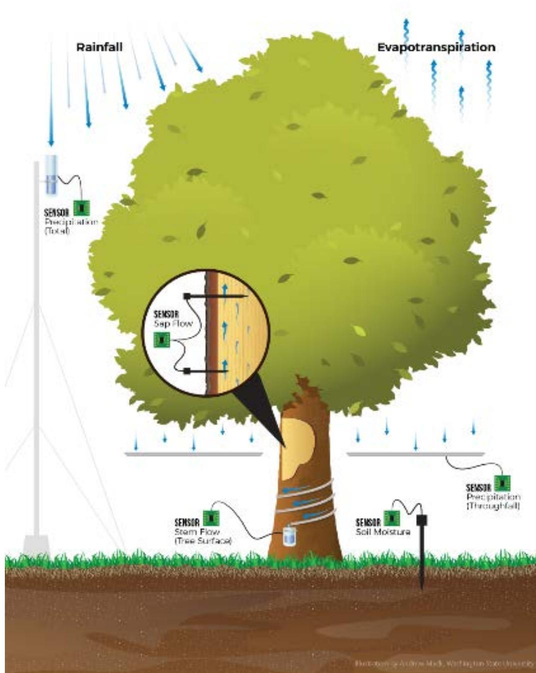
Figure 5: Sensor deployment strategy designed to quantify interception and transpiration
