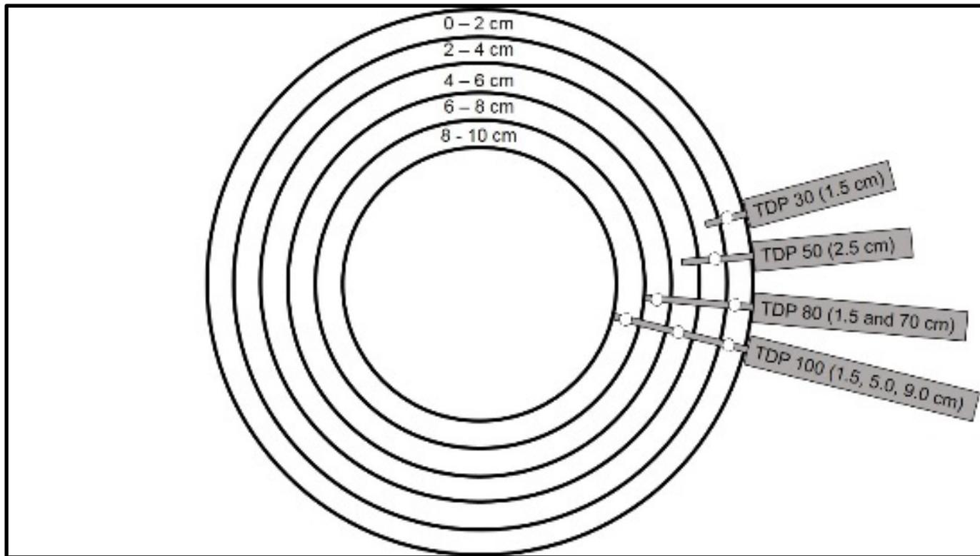
Figure 8: Figure TDP. Radial depth bands of sap flow rates are computed from data collected from TDP sensors. Open circles indicate locations of thermocouples. Very little flow (or none) occurs at depths exceeding 9.0 cm for most tree species.
