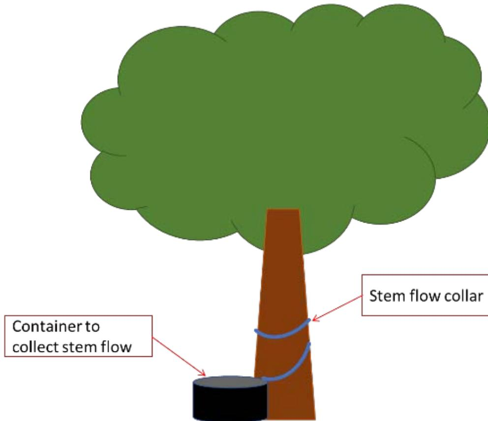
Figure 7: Profile of view showing arrangement of stem flow collar and stem flow container
