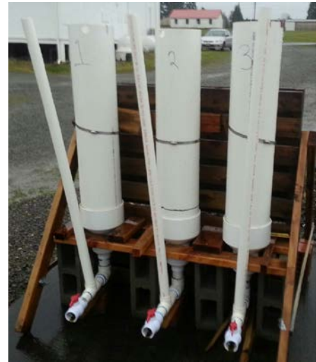
Figure 1: Surrogate columns for destructive soil layer sampling.
