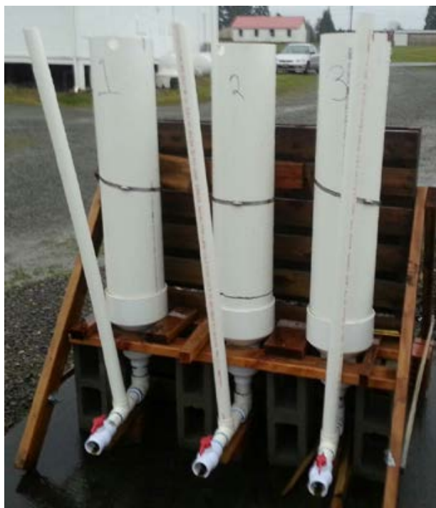
Figure 1. Surrogate columns for conditioned toxicity testing and destructive soil layer sampling.
