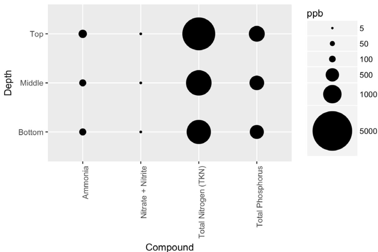
Figure 4: Concentrations of nutrient parameters in µg/kg (ppb) in the top (0-15 cm), middle (15-30 cm), and bottom (30-40 cm) strata of triplicate soil columns after clean water conditioning/ $K_{sat}$  testing.
