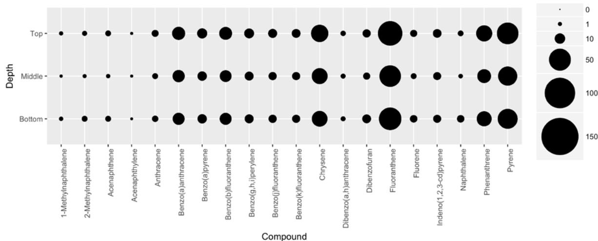
Figure 3: Concentrations of tested PAH congeners in µg/kg (ppb) in the top (0-15 cm), middle (15-30 cm), and bottom (30-40 cm) strata of triplicate soil columns after clean water conditioning/ $K_{sat}$  testing.
