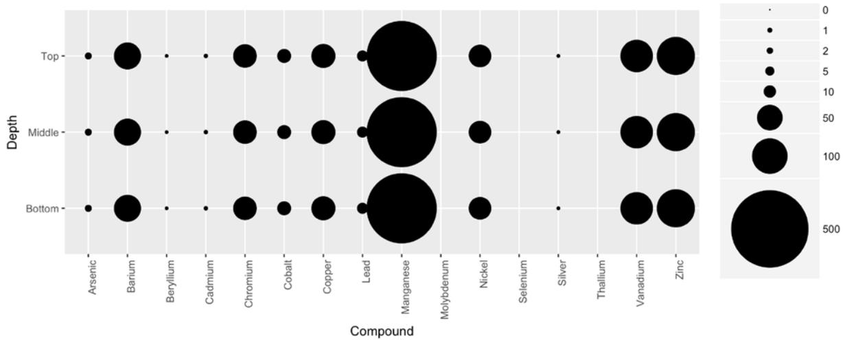
Figure 2: Metal concentrations in µg/kg (ppb) in the top (0-15 cm), middle (15-30 cm), and bottom (30-40 cm) strata of triplicate soil columns after clean water conditioning/ $K_{sat}$  testing.
