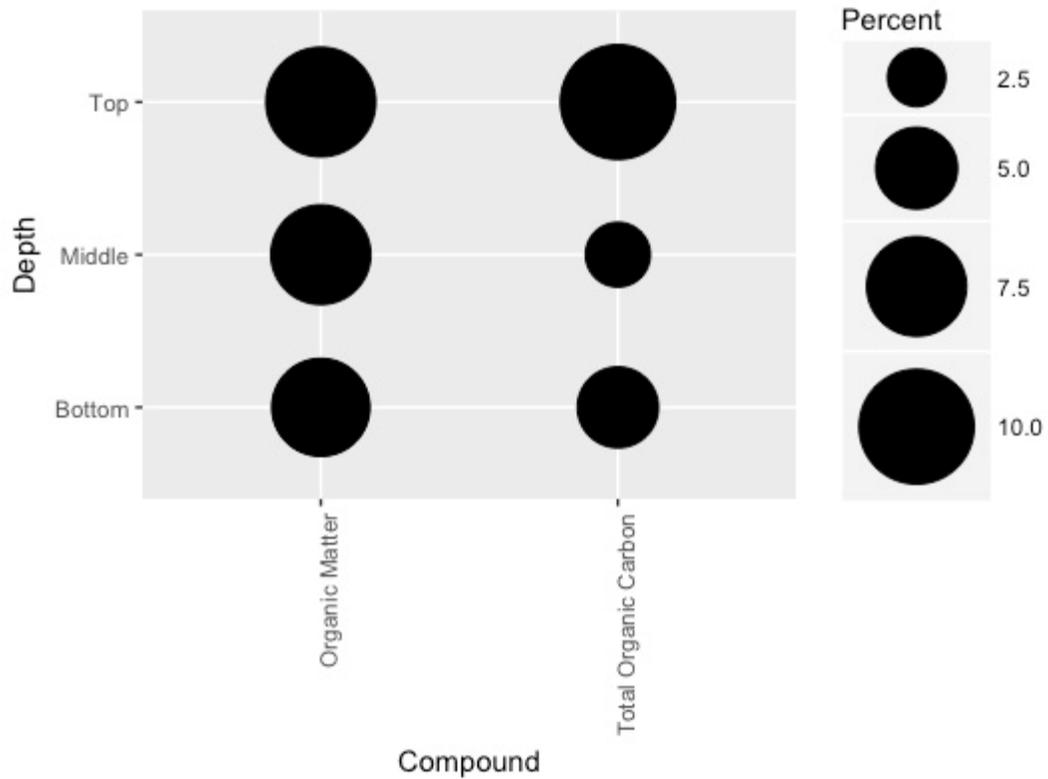
Figure 5: Concentrations of selected conventional parameters expressed as percent of total mass in the top (0-15 cm), middle (15-30 cm), and bottom (30-40 cm) strata of triplicate soil columns after clean water conditioning/ $K_{sat}$  testing.
