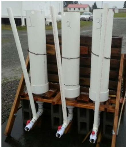
Figure 1: (Above) Field test site including vertical standpipes for  $K_{sat}$  testing. (Below) Surrogate columns for destructive soil layer sampling.
