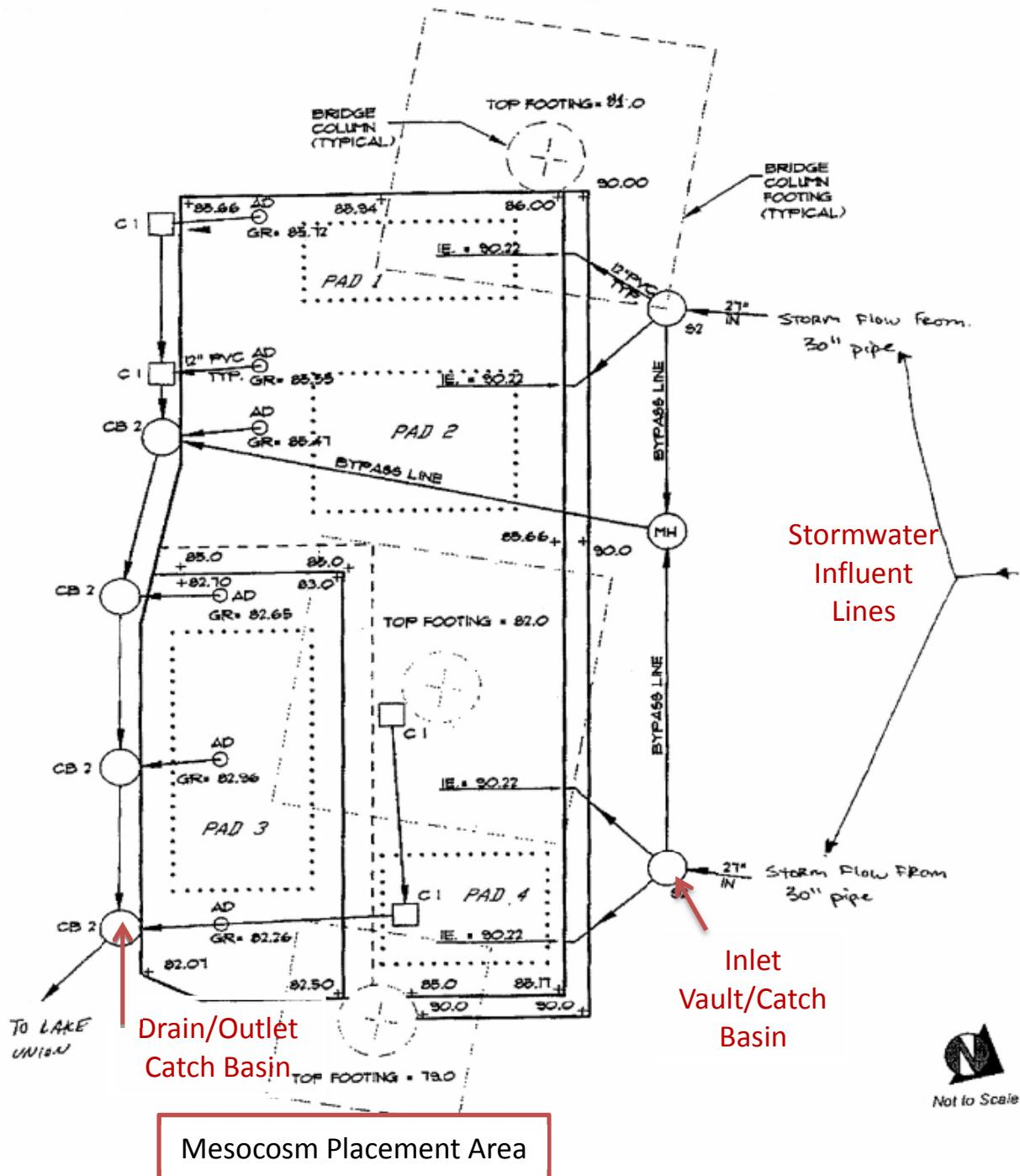
Figure 1. Layout of WSDOT Ship Canal Stormwater Research Facility with vault inlet-drain lines shown. See Figure 3 for pump piping
