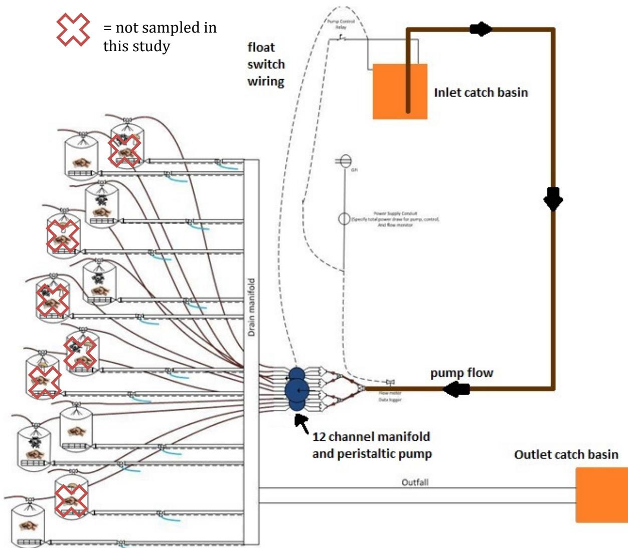
**Figure 2.** Schematic of Mesocosm Placement Area; mesocosms not sampled during this study are part of the Taylor et al. (2016) study.
