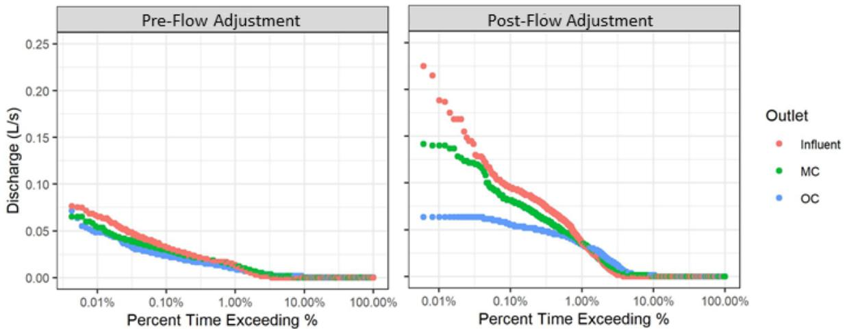
Figure 3-13 Flow Duration Curve for Mesocosms with New Standard BSMs
