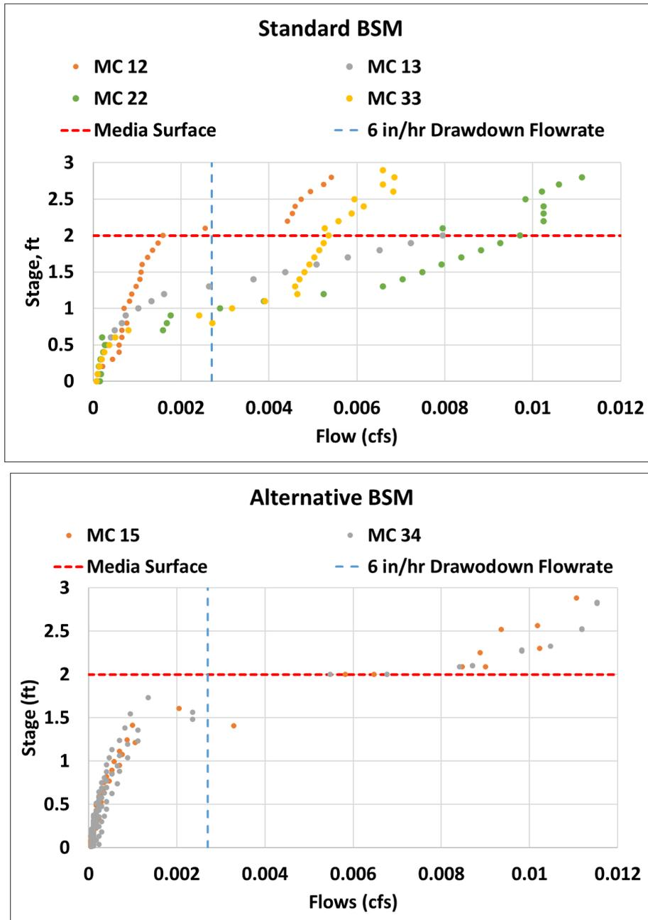
Figure 3-4 Stage-discharge Relationships of Media-Controlled Mesocosms
