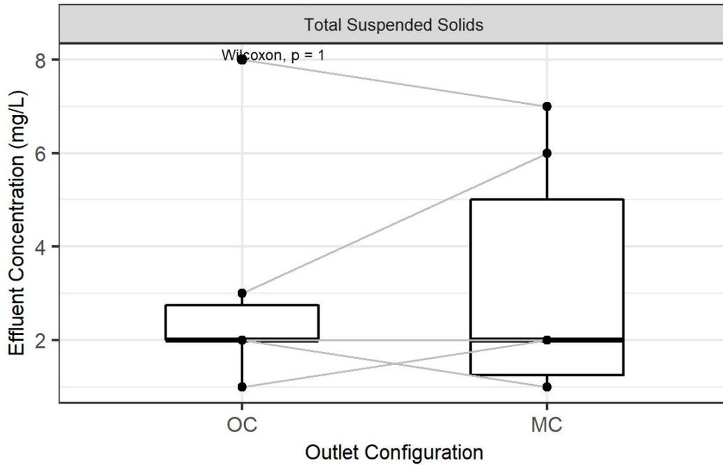
Figure A14: Mature Standard BSM: Comparison of Effluent Concentration between Outlet-Controlled and Media-Controlled Mesocosms for Total Suspended Solids
