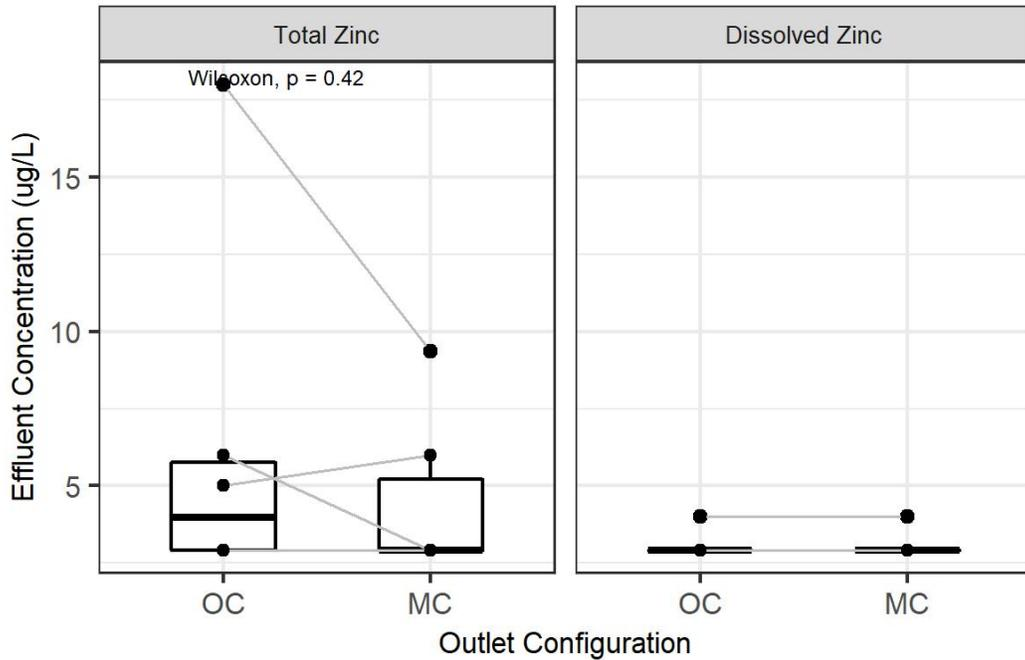
Figure A4: Alternative BSM: Comparison of Effluent Concentration between Outlet-Controlled and Media-Controlled Mesocosms for Total and Dissolved Zinc. Dissolved Zinc in several effluent samples across both treatments were listed as non-detect - therefore numerically identical. The Wilcoxon Signed-Rank test could not be evaluated.
