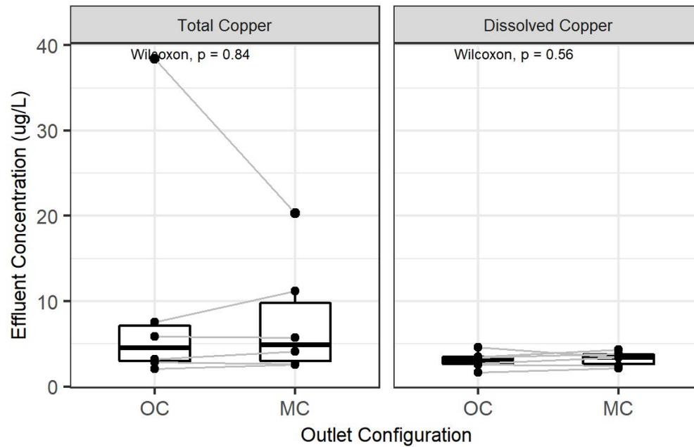
Figure A1: Alternative BSM: Comparison of Effluent Concentration between Outlet-Controlled and Media-Controlled Mesocosms for Total and Dissolved Copper
