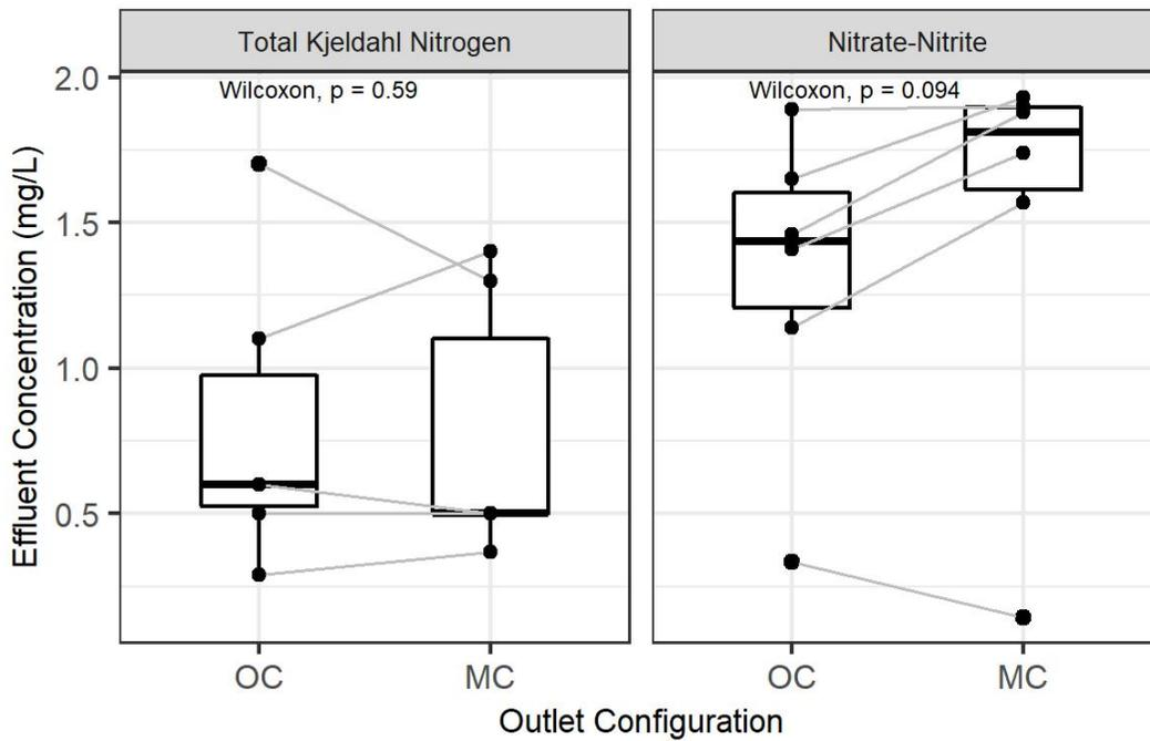
Figure A7: Alternative BSM: Comparison of Effluent Concentration between Outlet-Controlled and Media-Controlled Mesocosms for Nitrogen
