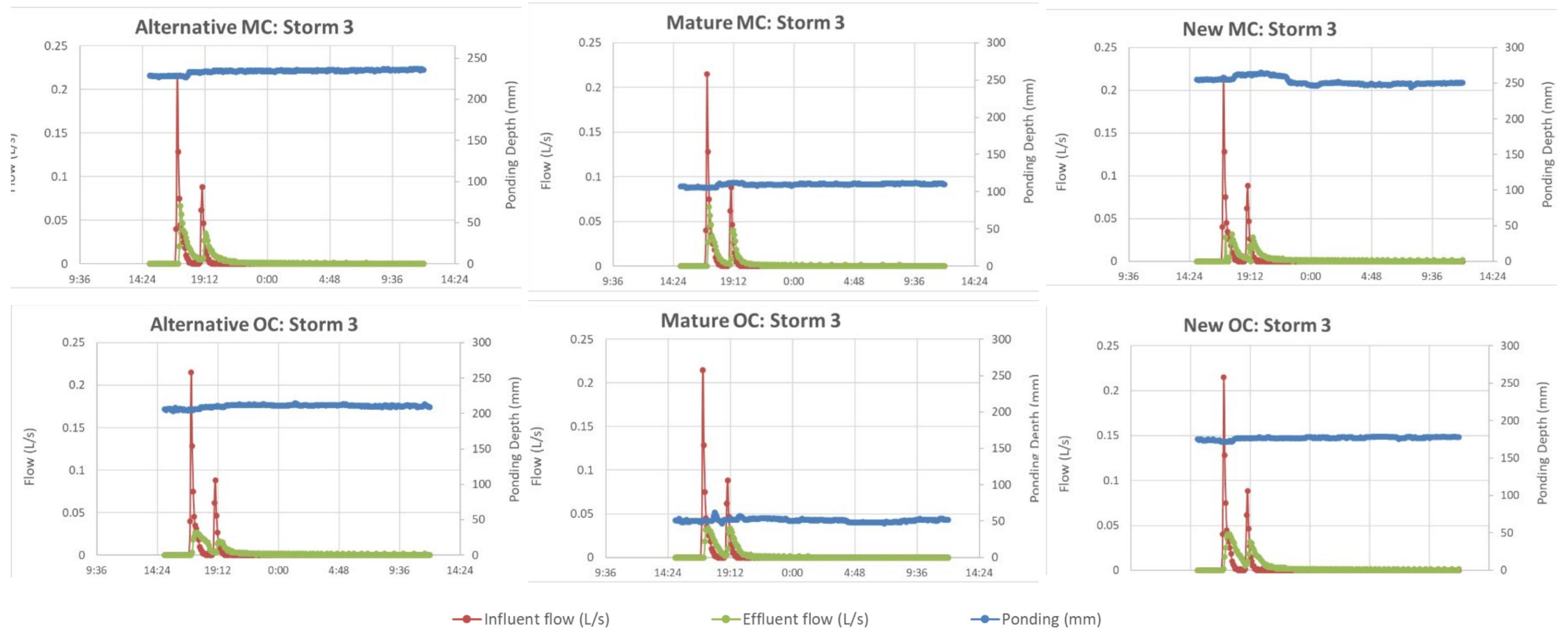
Figure 3-10 Inflow, outflow, and ponding level in six mesocosms during a natural storm (5/27 – 5/29, 2022)
