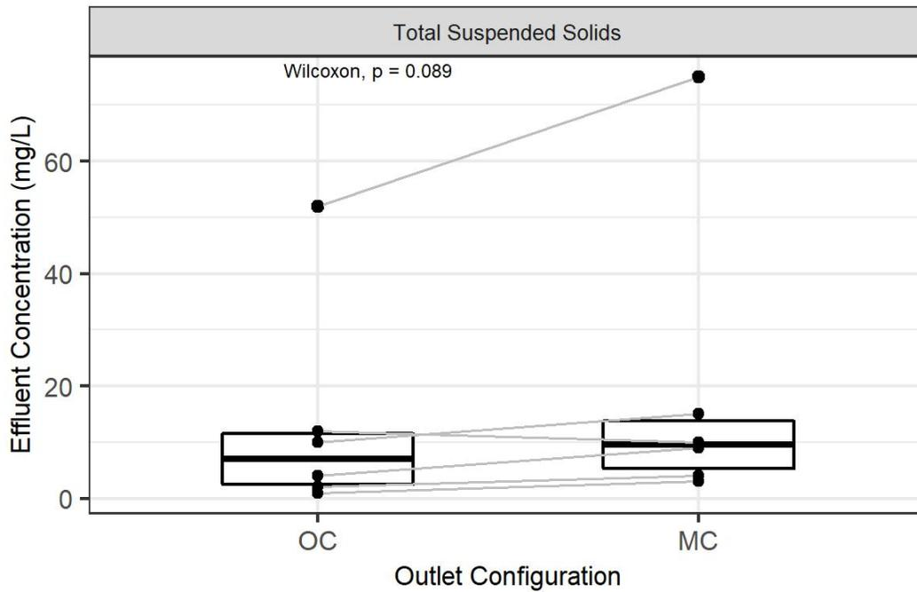
Figure A13: Alternative BSM: Comparison of Effluent Concentration between Outlet-Controlled and Media-Controlled Mesocosms for Total Suspended Solids
