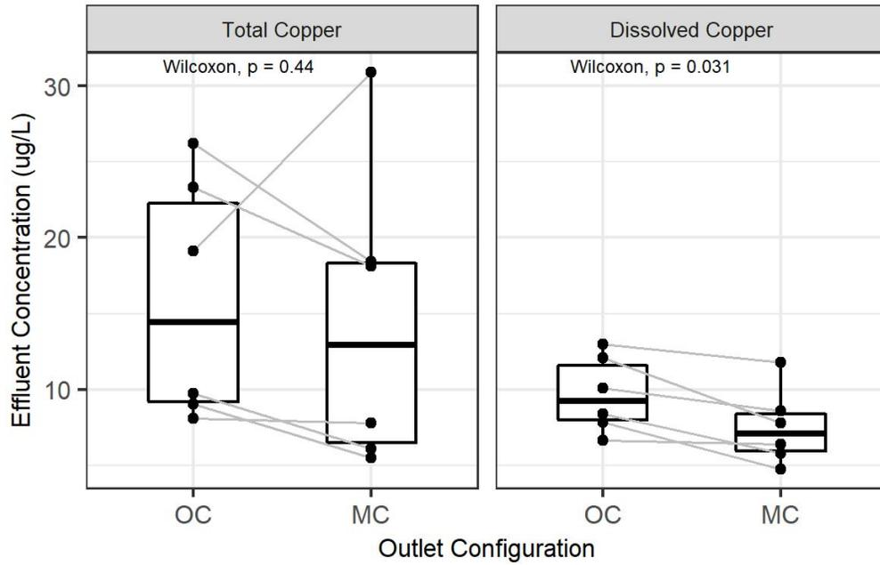
Figure A3: New Standard BSM: Comparison of Effluent Concentration between Outlet-Controlled and Media-Controlled Mesocosms for Total and Dissolved Copper
