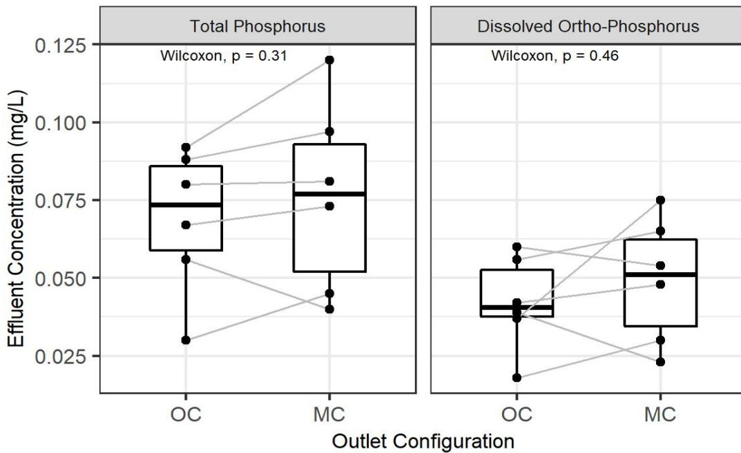
Figure A11: Mature Standard BSM: Comparison of Effluent Concentration between Outlet-Controlled and Media-Controlled Mesocosms for Phosphorus
