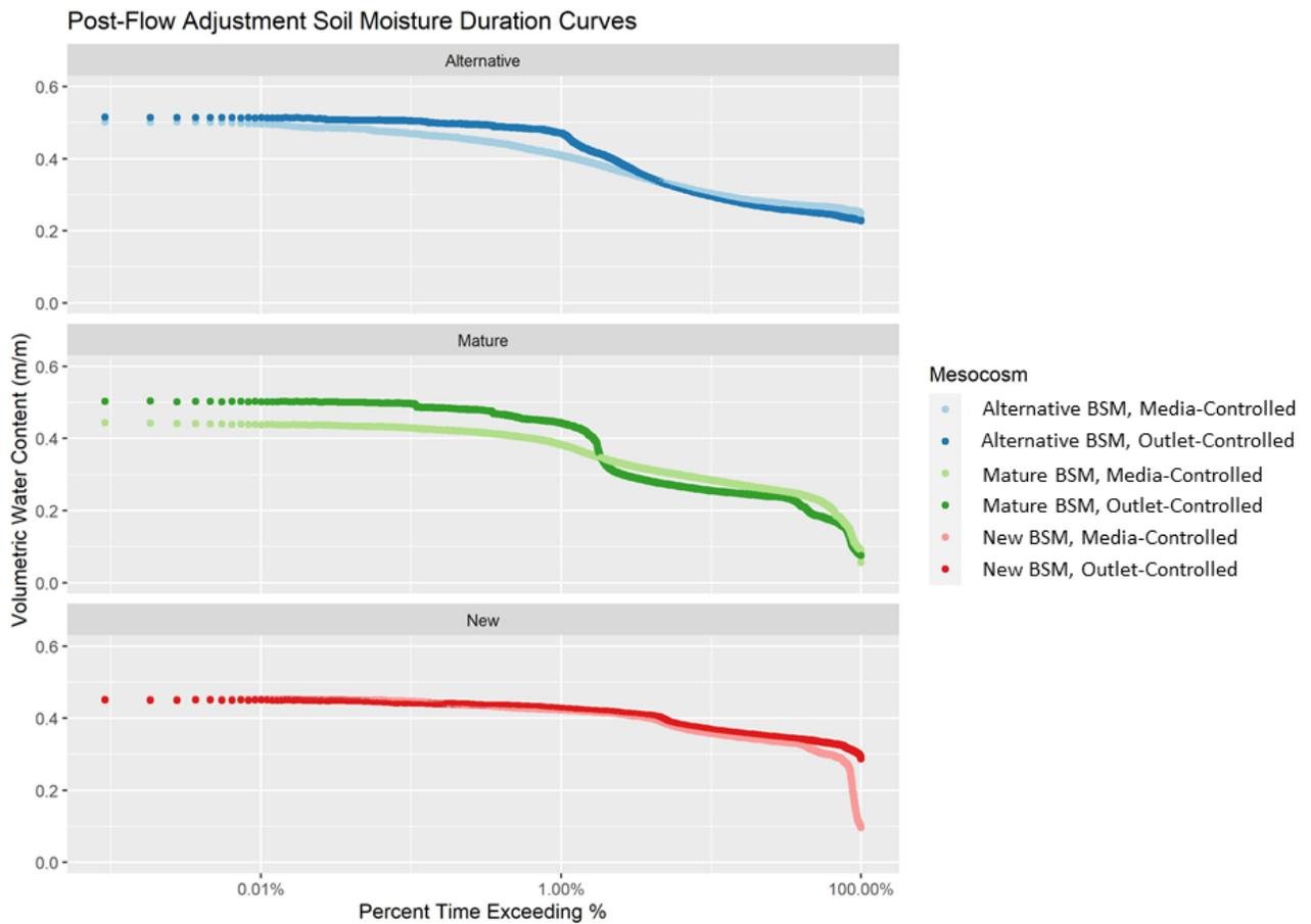
*Figure 3-6 Post-Flow Adjustment Period Soil Moisture Duration Curves for Mesocosms grouped by BSM Type*
