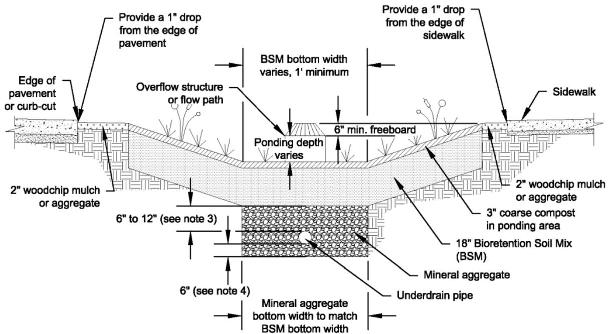
Figure 1-1: Typical design schematic for bioretention swale from 2019 SWMMWW.
