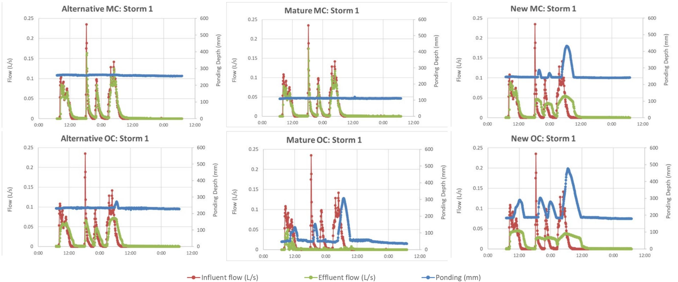
Figure 3-8 Inflow, outflow, and ponding level in six mesocosms during a natural storm (5/6 – 5/8, 2022)
