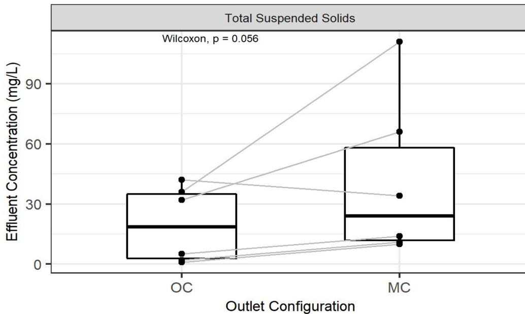
Figure A15: New Standard BSM: Comparison of Effluent Concentration between Outlet-Controlled and Media-Controlled Mesocosms for Total Suspended Solids
