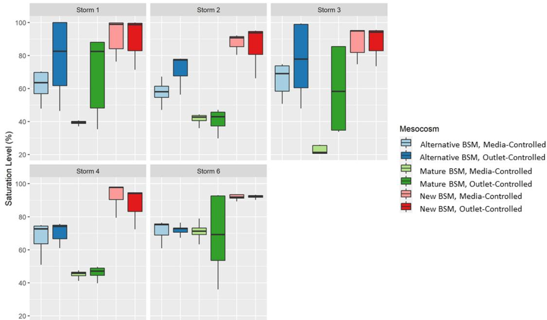
Figure 3-7 Soil Saturation Levels during Water Quality Testing (Synthetic Storm) Events
