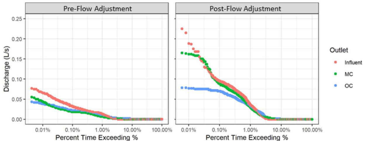
Figure 3-11 Flow Duration Curve for Mesocosms with Alternative BSMs
