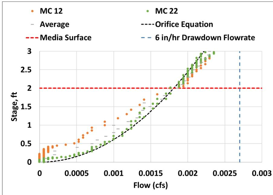
*Figure 3-3 Stage-Discharge Relationships of Outlet-Controlled Mesocosms*
