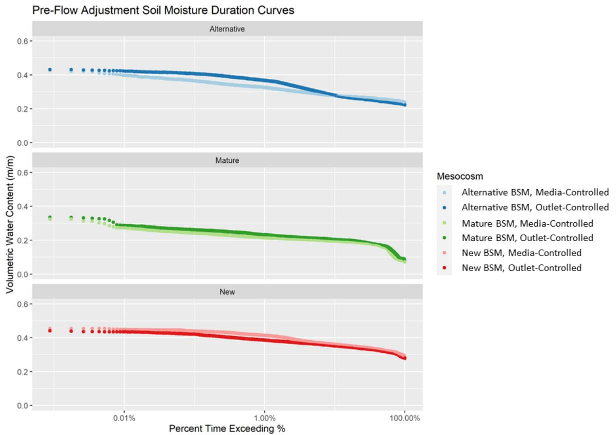
Figure 3-5 Pre-Flow Adjustment Period Soil Moisture Duration Curves for Mesocosms grouped by BSM Type
