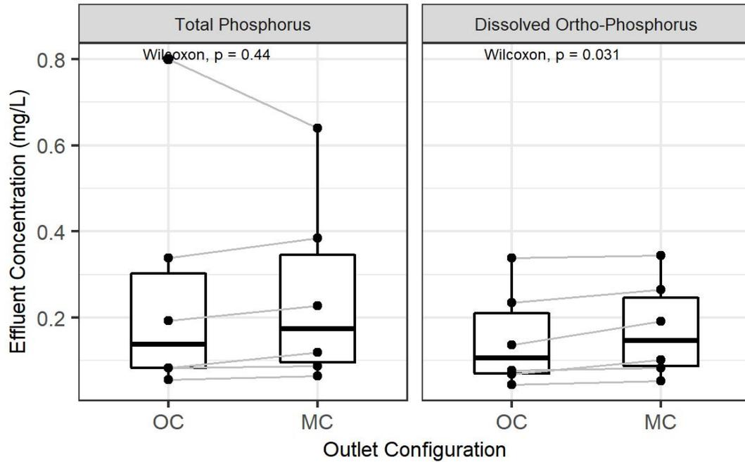
Figure A10: Alternative BSM: Comparison of Effluent Concentration between Outlet-Controlled and Media-Controlled Mesocosms for Phosphorus
