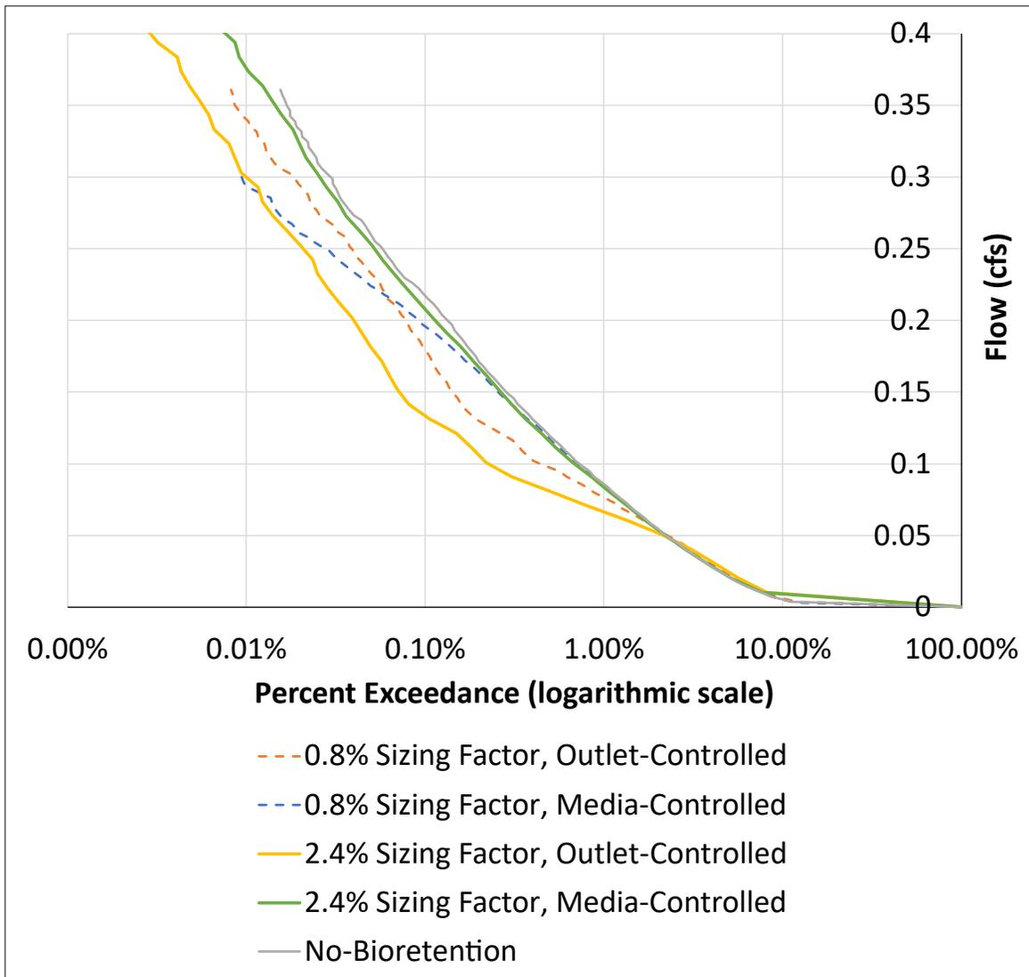
Figure 3-14. Flow Duration Curves Comparison between Media-Controlled and Outlet-Controlled in 0.8% and 2.4% Sizing Scenarios (Standard BSM, 0.1 in/hr Native Soil Infiltration Rate).
