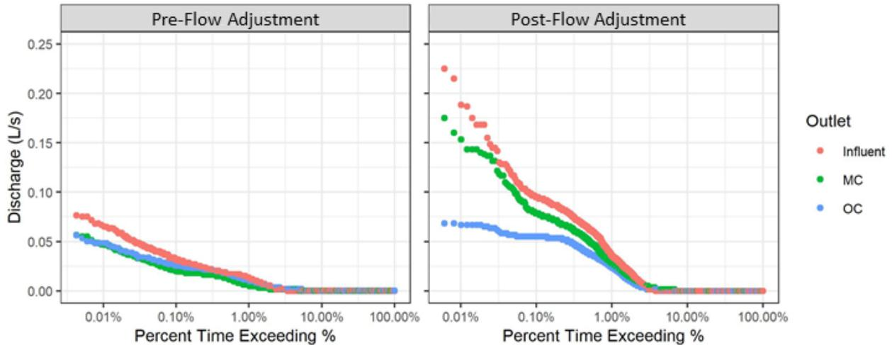
Figure 3-12 Flow Duration Curve for Mesocosms with Mature Standard BSMs
