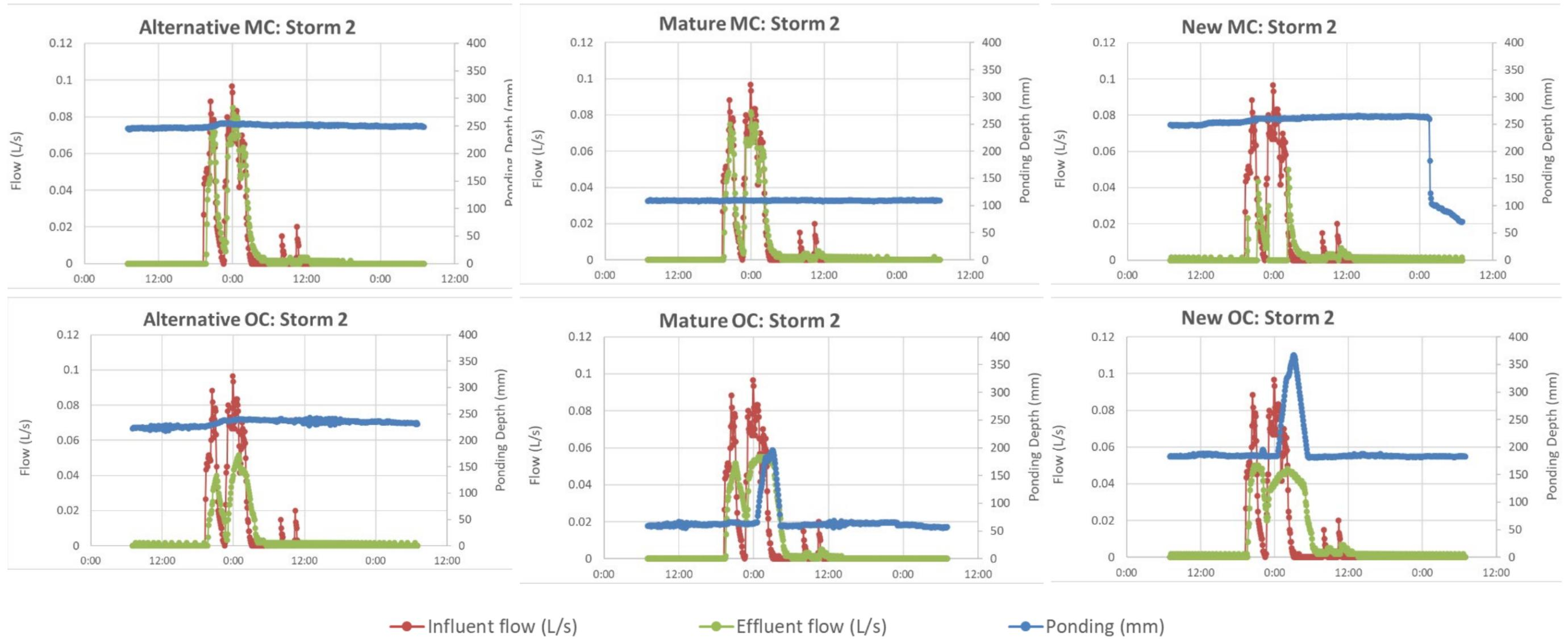
Figure 3-9 Inflow, outflow, and ponding level in six mesocosms during a natural storm (6/4 – 6/6, 2022)
