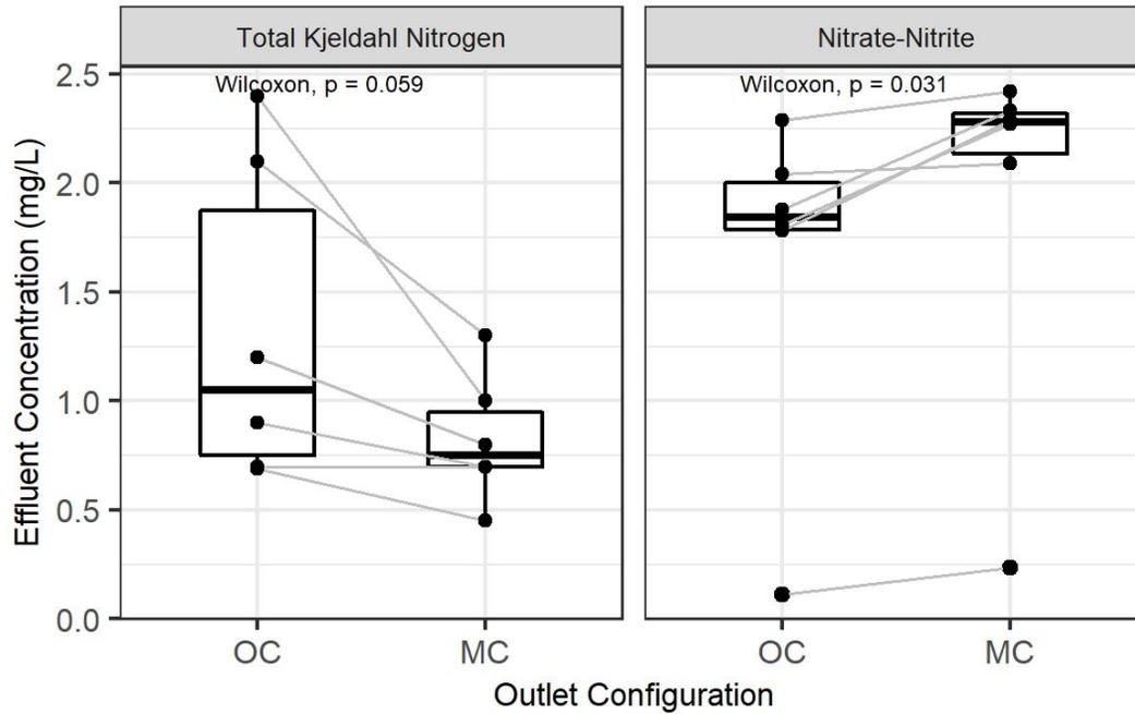
Figure A8: Mature Standard BSM: Comparison of Effluent Concentration between Outlet-Controlled and Media-Controlled Mesocosms for Nitrogen
