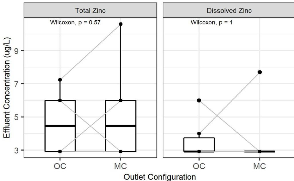
Figure A5: Mature Standard BSM: Comparison of Effluent Concentration between Outlet-Controlled and Media-Controlled Mesocosms for Total and Dissolved Zinc
