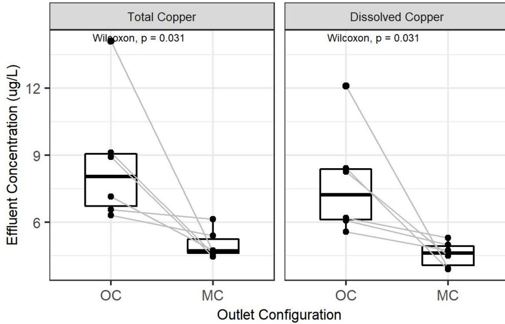
Figure A2: Mature Standard BSM: Comparison of Effluent Concentration between Outlet-Controlled and Media-Controlled Mesocosms for Total and Dissolved Copper
