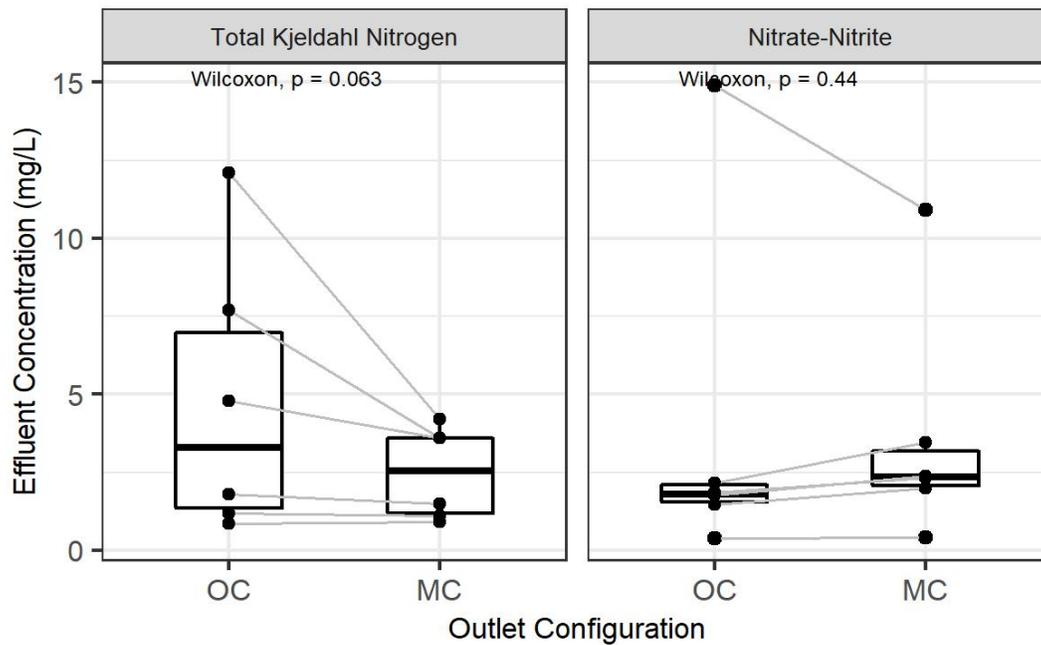
Figure A9: New Standard BSM: Comparison of Effluent Concentration between Outlet-Controlled and Media-Controlled Mesocosms for Nitrogen
