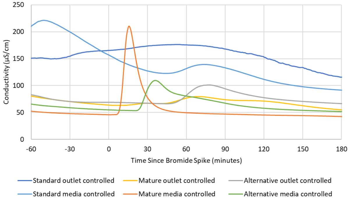
Figure 3-1 Example of Mesocosm Effluent Electrical Conductivity Monitoring Results during Event 2
