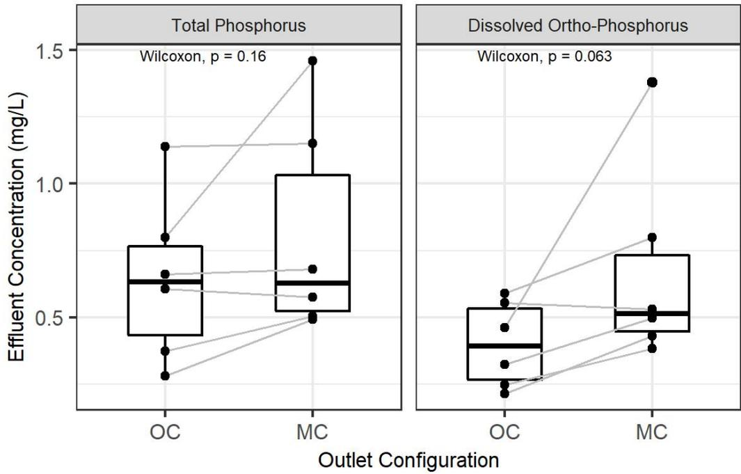
Figure A12: New Standard BSM: Comparison of Effluent Concentration between Outlet-Controlled and Media-Controlled Mesocosms for Phosphorus
