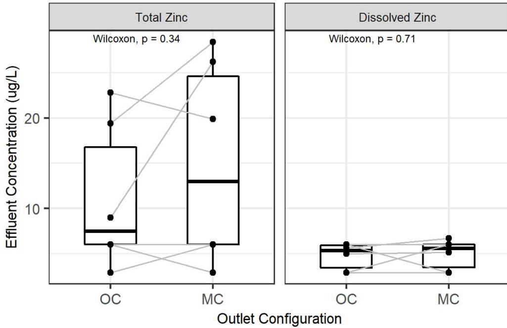
Figure A6: New Standard BSM: Comparison of Effluent Concentration between Outlet-Controlled and Media-Controlled Mesocosms for Total and Dissolved Zinc
