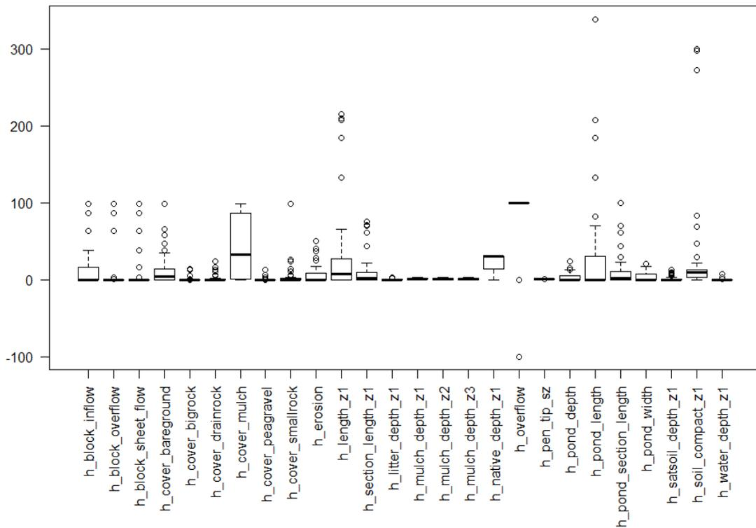
**Figure 4:** Boxplot showing the variability of all hydrology-related metrics' values at all sites aggregated across all zones of the bioretention cell/rain garden. Very few of the metrics produced normally distributed of data (i.e. bell curves) and the vast majority of data points for most metrics were at or near zero (i.e. Poisson distribution).<sup>2</sup>
