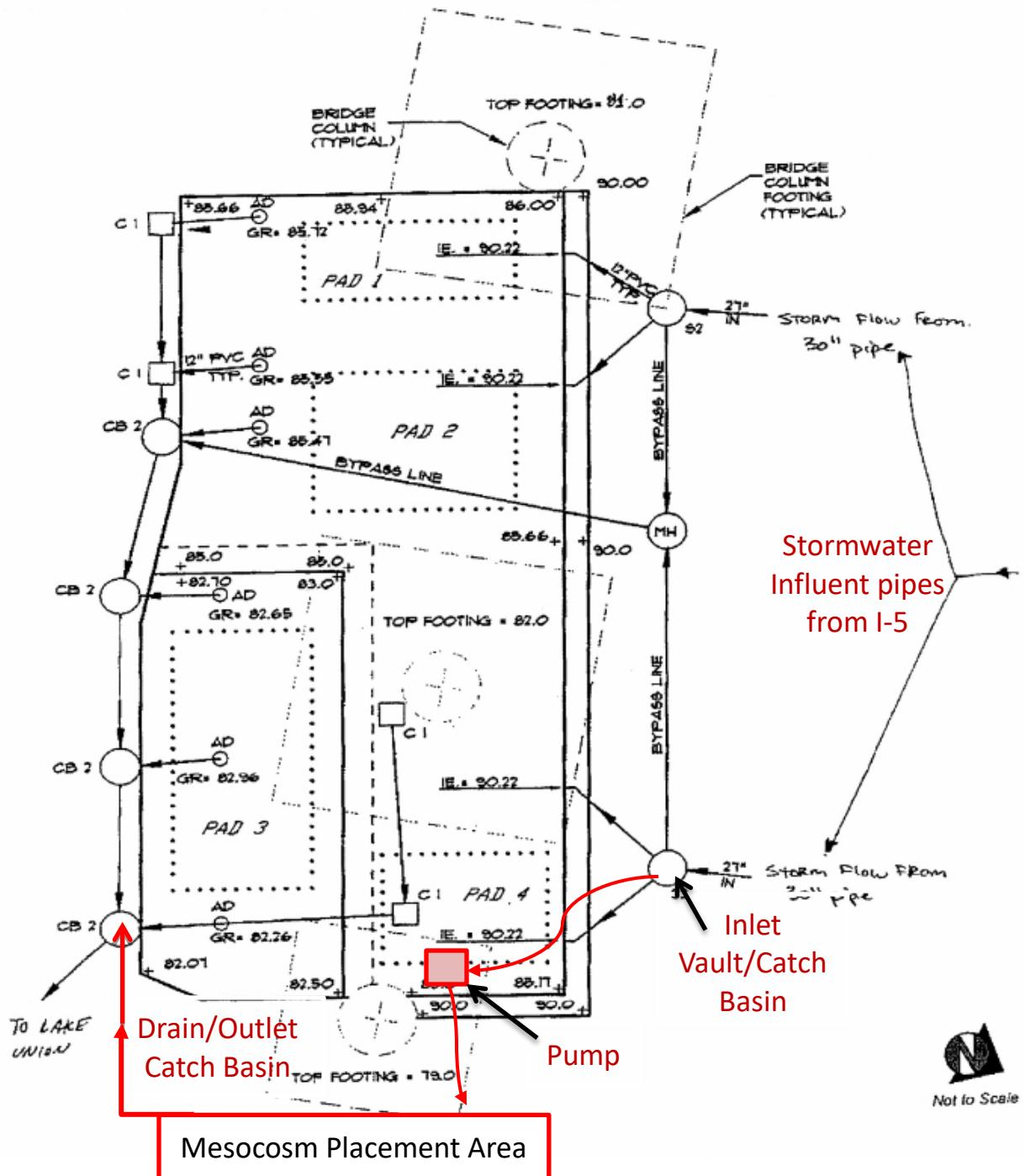
Figure 1. Layout of WSDOT I-5 Ship Canal Stormwater Research Facility with vault inlet-drain lines shown. See Figure 2 for additional pump piping information.
