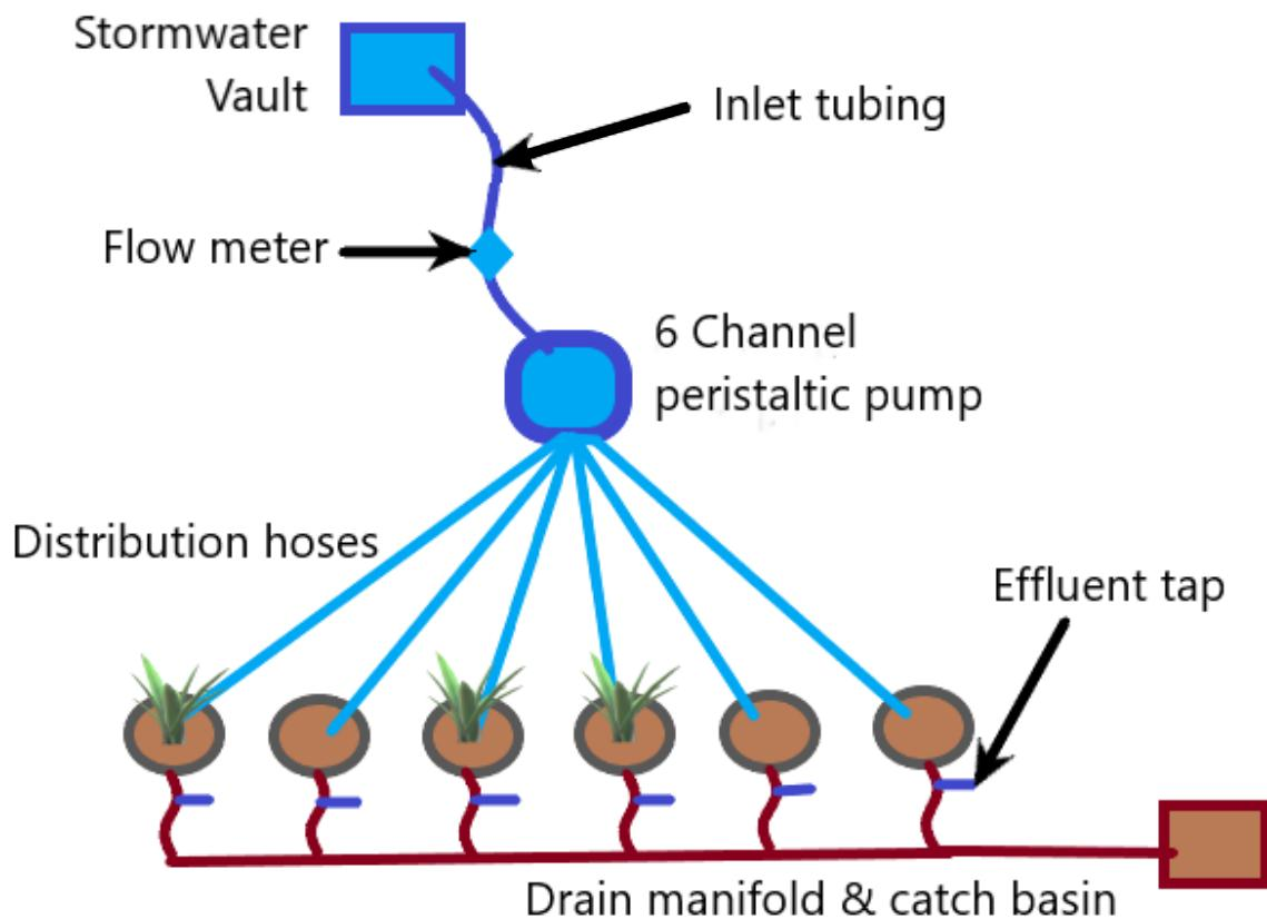
**Figure 3. Schematic of Mesocosm Placement Area with bare and planted mesocosms each sampled in triplicate.**
