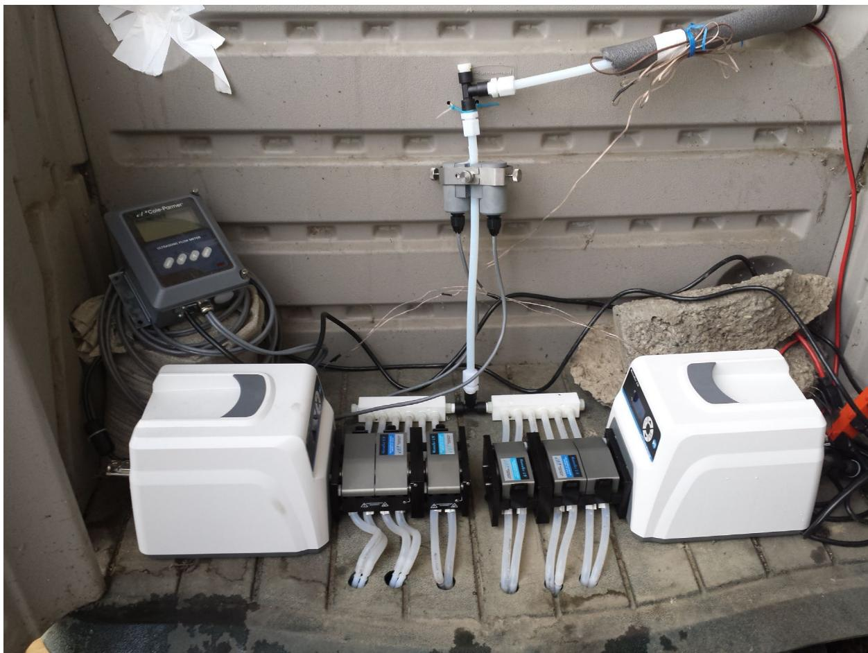
**Figure 4. Sampling pumps with distribution manifold and flow totalizer.**
