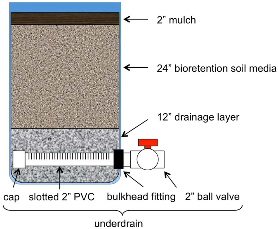
**Figure 1.** Diagram of bioretention unit using 55-gallon drum.
