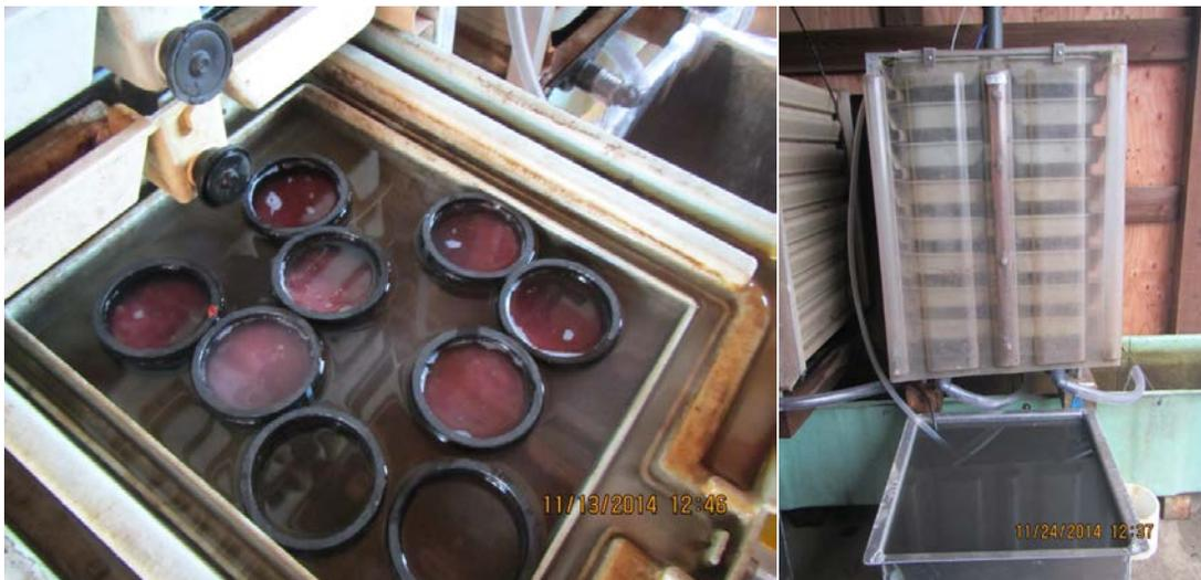
**Figure 5.** Embryo cups on a tray in the heath stack (left). Heath stack showing sump filled with 100% unfiltered runoff (right).
